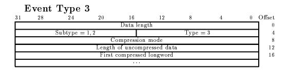
Figure C.6: Event structure type 3 (compressed)
