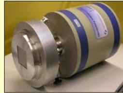
2D  $\mu$ -strip Si(Li) detector for Compton polarimetry.
