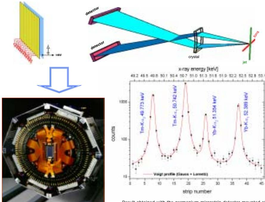
Result obtained with the germanium microstrip detector mounted at the FOCAL crystal spectrometer. The intensity pattern as function of the position (energy) identifies well resolved the two components of the Ka-doublet of Tm as well as those of Yb [2].
