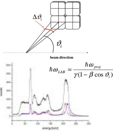
For a conventional detector the shift would result in a considerable Doppler broadening. Segmentation of PSGD detectors allows for an event-by-event Doppler correction of the registered x-rays.
