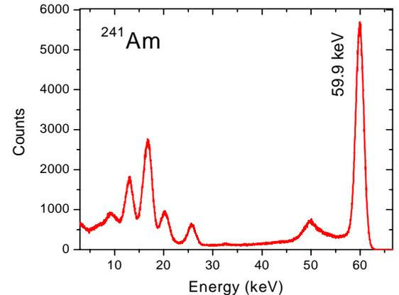
A sample photon spectrum recorded with one individual strip. For this purpose a standard  $^{241}\text{Am}$   $\gamma$ -ray source was used. The energy resolution achieved corresponds to 1.8 keV [FWHM] at 60 keV.
