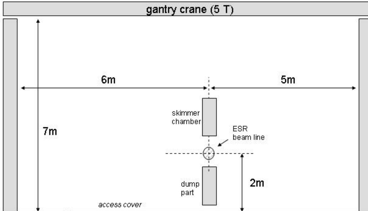
distance between beam pipe and the outer NESR concrete wall: 5 m
