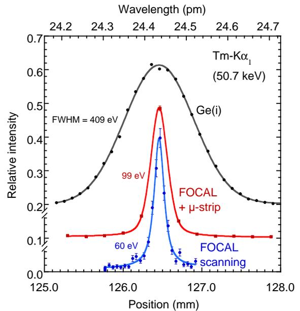
Figure 2: The wavelength profile of the  $\text{Tm-K}\alpha_1$  line measured as the pulse-height spectrum of a conventional solid-state Ge(i) detector or measured with the FOCAL spectrometer equipped either with a position-sensitive micro-strip detector or in scanning mode.
