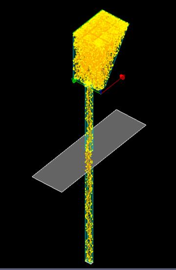
Step 6: Make generalization, instead of using phase space as a plane, one can use a bulk phase space cover the entire bar
