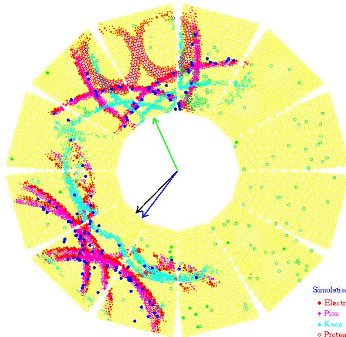
*Example: Comparison of real event to simulated response of DIRC to  $e/\pi/K/p$ .*
