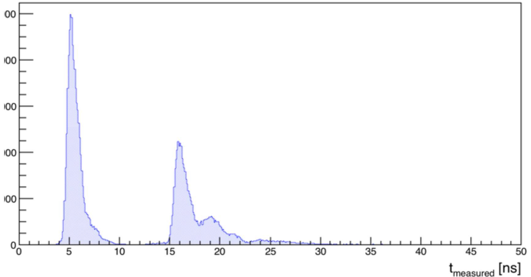
Detected Cherenkov photons time at 90 degree polar angle
