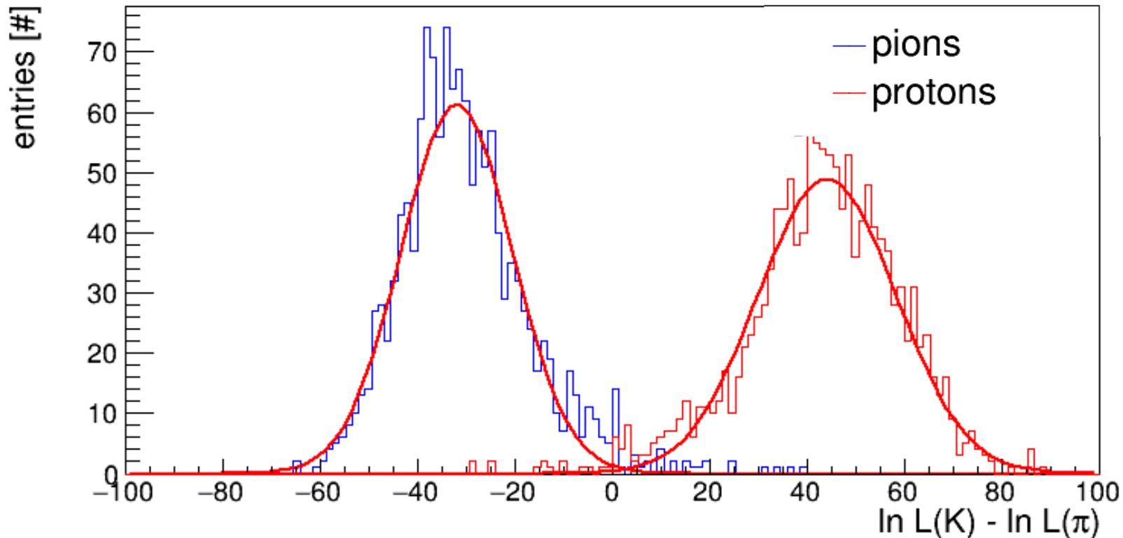
Proton-Pion log-likelihood difference distributions using time-based imaging
