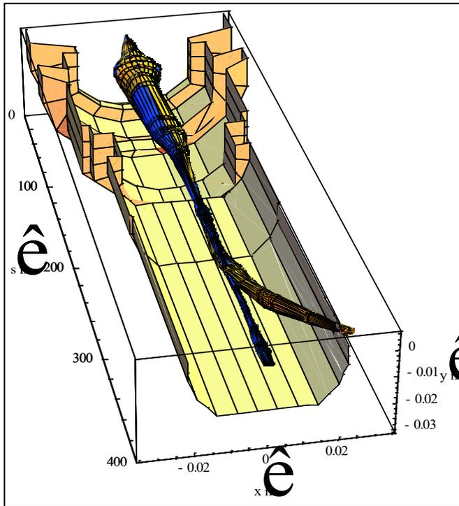
Secondary  $\text{Pb}^{81+}$  beam (25 W at design luminosity) emerging from IP and impinging on beam screen. Hadronic shower into superconducting coils can quench magnet.
