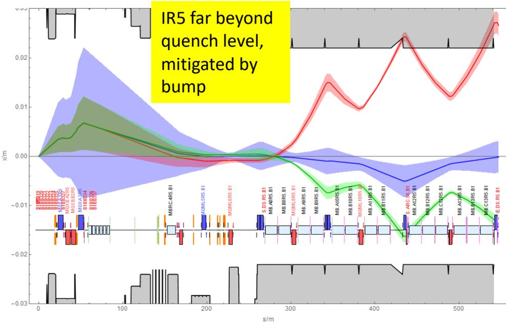
Bumps were adjusted empirically, good agreement with calculation, except left of IP5, location of 2015 BFPP quench test.
