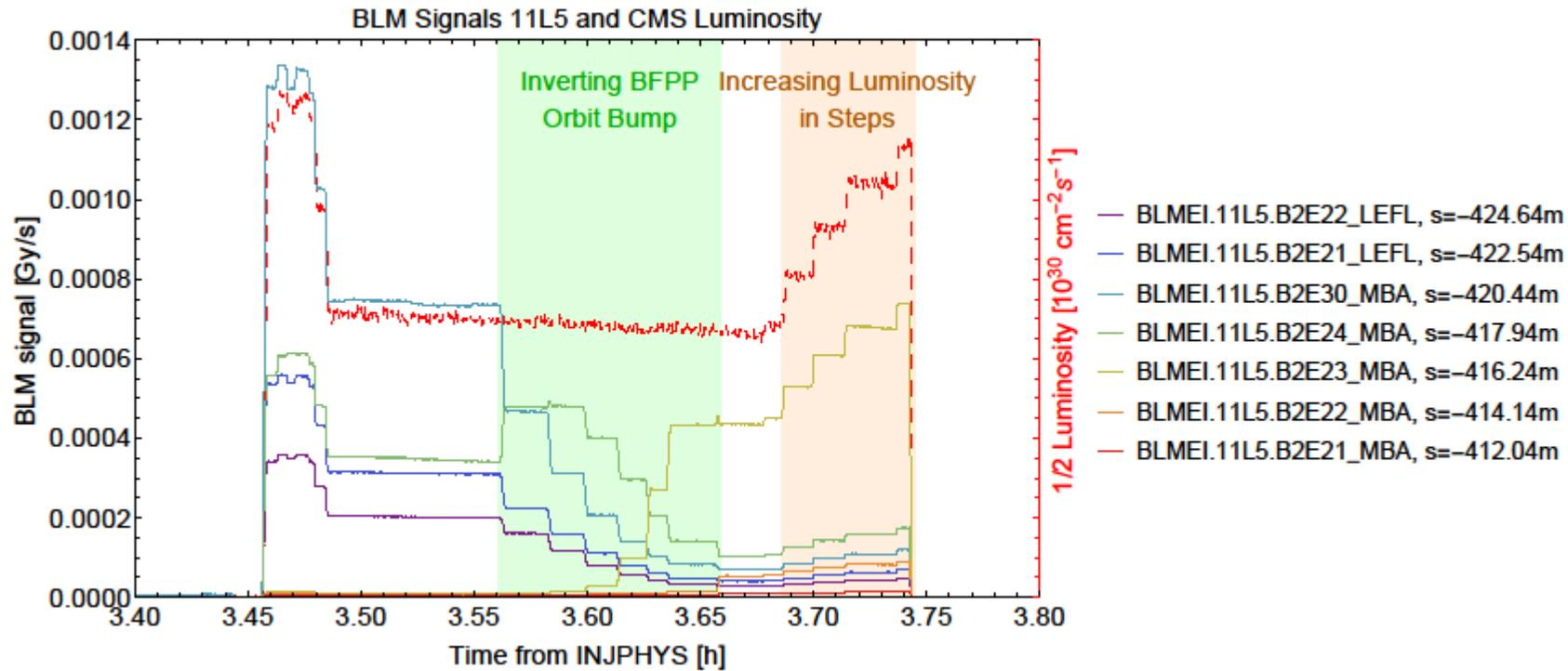
Intended to resolve decades of uncertainty about steady-state quench level of LHC dipole magnets. But some uncertainties in interpretation because of chamber misalignment in this particular DS.L5. Later a second collimation quench test with Pb was also successful.
