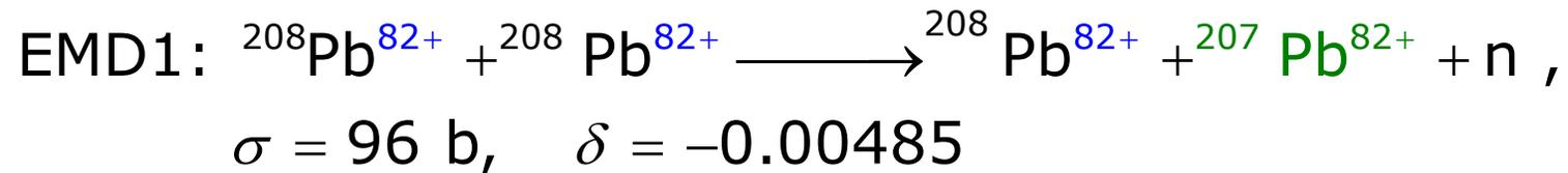
Each of these makes a secondary beam emerging from the IP with rigidity change that may quench bending magnets.
