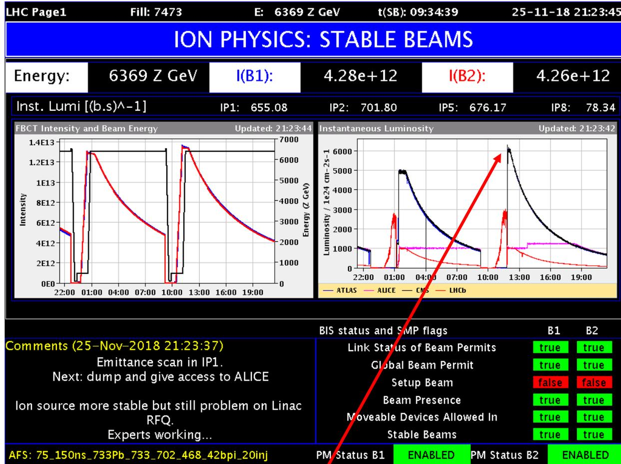
Comparison of BFPP losses with dump thresholds (specially set in BFPP loss zones) shows that we can go considerably further.
