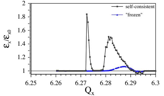
**FIGURE 2.** 2D simulation of KV distribution with  $\Delta Q_x = 0.045$  and octupole (100 A) as function of bare machine tune, showing self-consistent and “frozen-in” models (after 1000 turns).
