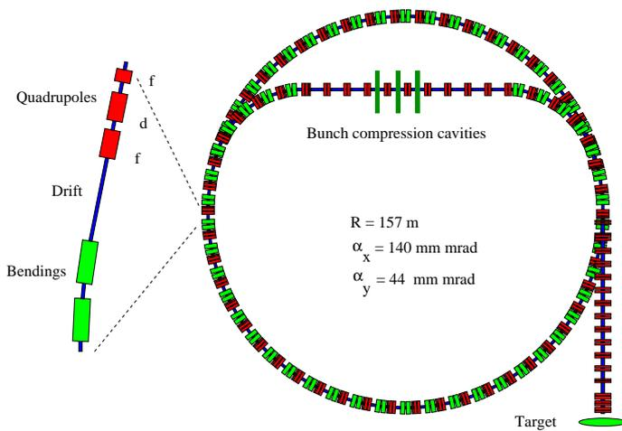
Figure 1: SIS100 lattice for fast compression scheme.
