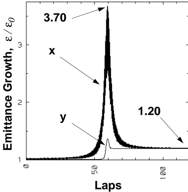
Figure 2: RMS emittance growth versus ring laps of the bunch centroid for SIS18.
