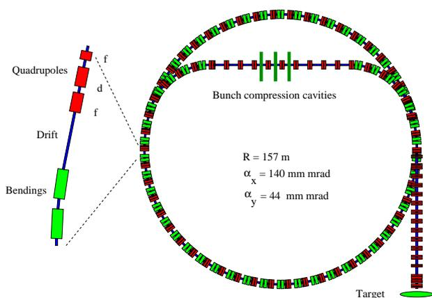
Figure 1: Lattice example of a 100 Tm synchrotron for plasma physics applications to reach 100 eV in solid Au using  $10^{13}$   $U^{4+}$  ions at 127 MeV/u.
