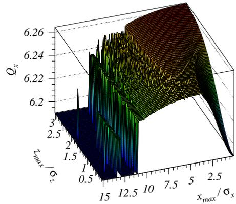
**FIGURE 3.** Nonlinear tune  $Q_x$  as function of the maximum initial amplitude ( $x_{max}, z_{max}$ ) for  $Q_{x0} = 6.265$ . The longitudinal motion is frozen.
