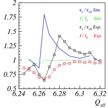
**FIGURE 4.** Final beam emittance (solid) and intensities (dashed) versus working point in simulations (no markers) up to  $1.5 \times 10^5$  turns and experiment (markers) up to  $4.4 \times 10^5$ .
