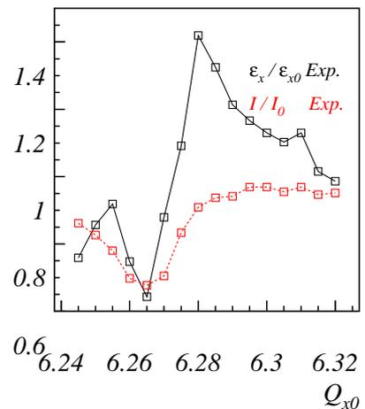
**FIGURE 1.** Experimental findings: normalized final emittance and beam intensity as function of the working point.
