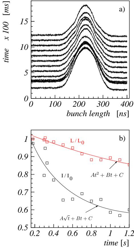
**FIGURE 2.** Measurements at  $Q_{x0} = 6.265, Q_{y0} = 6.12$ : a) Waterfall plot of the longitudinal profile as function of time; b) Beam intensity and bunch length as function of storage time. The solid lines are fitted with data by using the functional dependance reported.
