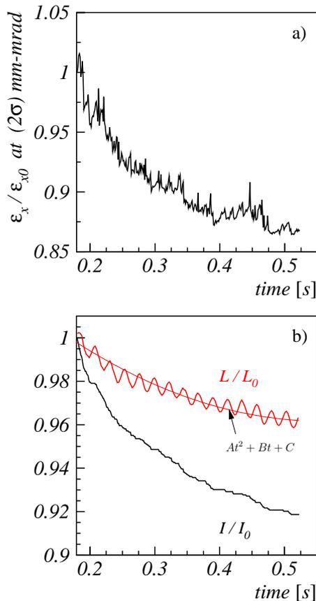
**FIGURE 6.** Simulation for  $Q_{x0} = 6.26$ : a) rms horizontal emittance versus time; b) beam intensity and bunch length with fitted curve as function of storage time.
