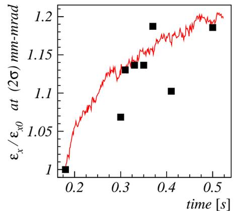
**FIGURE 5.** Comparison of emittance time evolution in measurements (markers) and simulation at  $Q_{x0} = 6.28$ .
