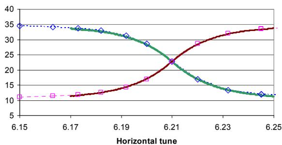
**FIGURE 4.** 3D simulation results (IMPACT code) in the case where the synchrotron period is much larger than the crossing time (full line), and fit (dotted line), using the numerical values of the measured case (see Fig. 2).
