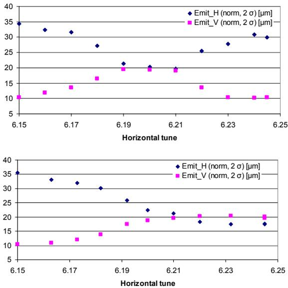
**FIGURE 2.** Measured intensity-dependent emittance transfer in 2003 for  $Q_y = 6.21$  (upper) in the static case (constant horizontal tune from injection to the measurement point), (lower) in the dynamic case (the horizontal tune was changed linearly from 6.15 to 6.25 in 100 ms).
