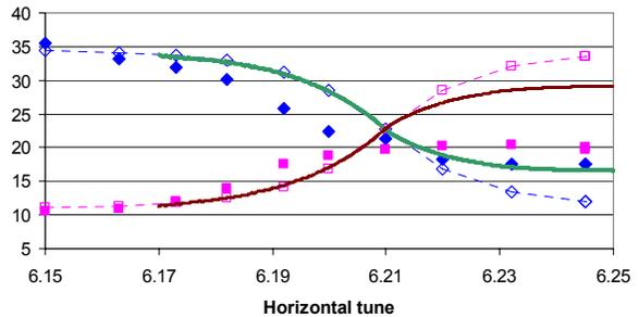
**FIGURE 5.** Measurements (dots, see Fig. 2), 3D simulation results (IMPACT code) in the real measured case where the synchrotron period is not much larger than the crossing time (full line), and fit of the 3D simulation results in the case where the synchrotron period is much larger than the crossing time (dotted line).
