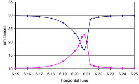
**FIGURE 2.** Simulated final emittances (mm mrad) for fixed  $Q_{0,y} = 6.21$  as function of  $Q_{0,x}$  (2D PIC with MICROMAP).
