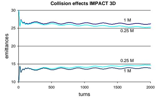
**FIGURE 4.** Emittances (mm mrad) for 1 M and 0.25 M simulation particles and  $Q_{0,x} = 6.19$  in IMPACT 3D.
