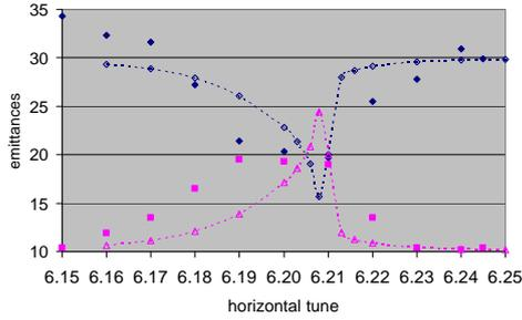
**FIGURE 3.** Final measured (full markers) and simulated (open markers) emittances for fixed  $Q_{0,y} = 6.21$  as function of  $Q_x$ .
