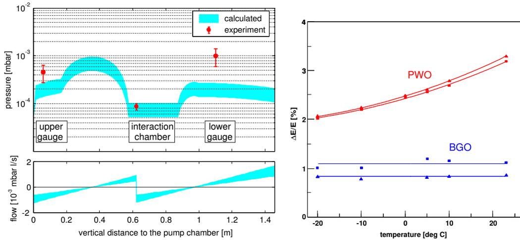
(a) Comparison of experimental (red points) and calculated vacuum (light blue band) in the target pipe of the PTS. The errors indicate a  $1\sigma$  uncertainty. The experimental points lie factors 2 to 4 above the calculated band but agree within  $2\sigma$ . The lower part shows the calculated gas flow, which is below zero if the gas flows to the left the figure and positive if the flow is to the right, i.e. upwards and downwards respectively at the experiment.
