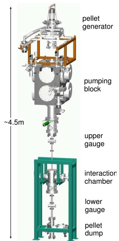
Figure 1: Pellet Test Station PTS designed for testing and further development of the target. On this drawing vacuum gauges, diagnostic tools, several pumps, and fittings are omitted.
