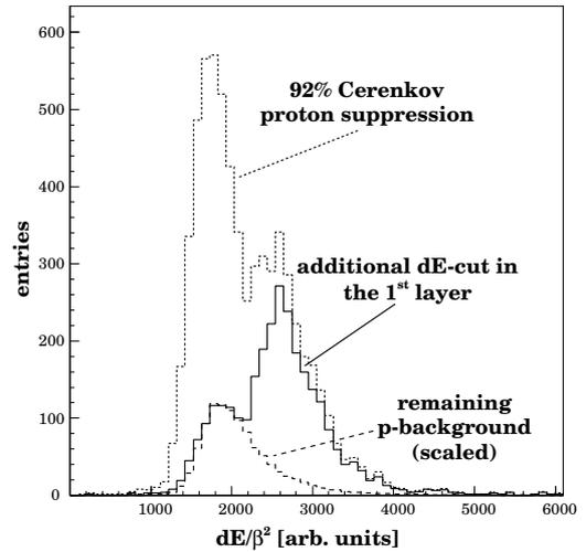
Fig. 2: Energy loss in the 2<sup>nd</sup> layer of the forward hodoscope (scaled with  $\beta_d^{-2}$ ) using only Č-suppression (dotted), dE-cut in the first layer (solid), proton contribution extrapolated by an active selection of these particles and scaled (dashed)
