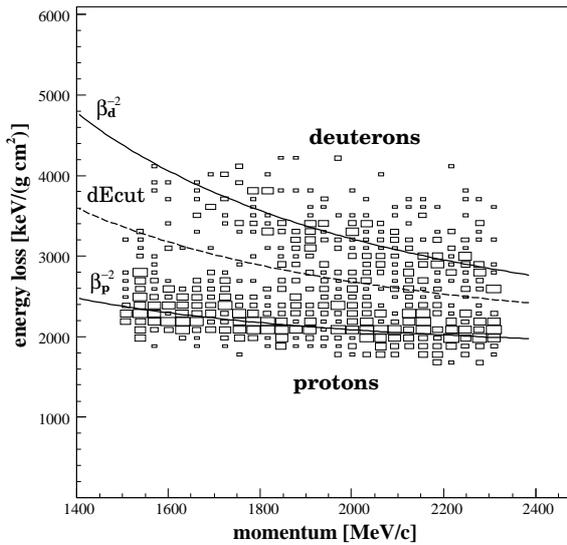
Fig. 1: Momentum dependent cut on the energy loss in the 1<sup>st</sup> layer of the forward hodoscope after 97% proton suppression; the bands from protons and deuterons can be approximated well by functions of  $\beta^{-2}$ .
