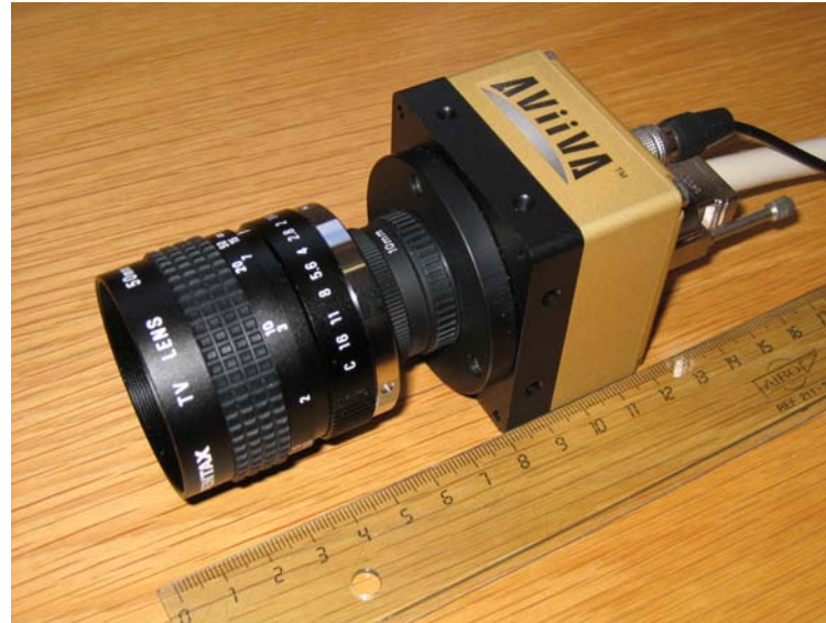
98 kHz, 512 pixel line-scan camera
