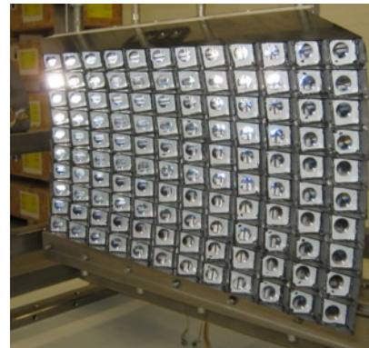
Barrel EMC alveoles and rear inserts
