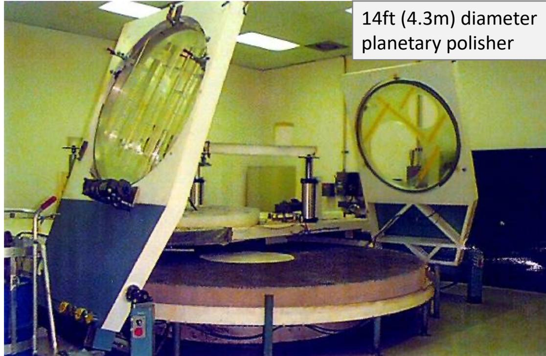
14ft (4.3m) diameter planetary polisher
