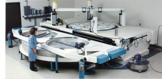
4.2m-diameter planetary polisher at InSync Inc (BABAR DIRC)
