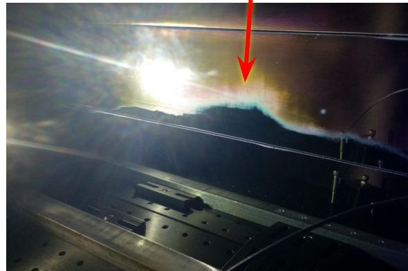
Type II anodized Al strongback in optical box. Coated with white cloudy residue after few months in water.
