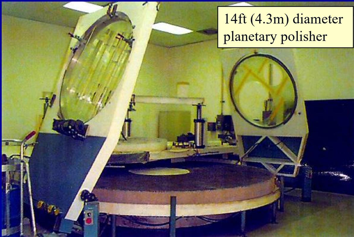
14ft (4.3m) diameter planetary polisher
