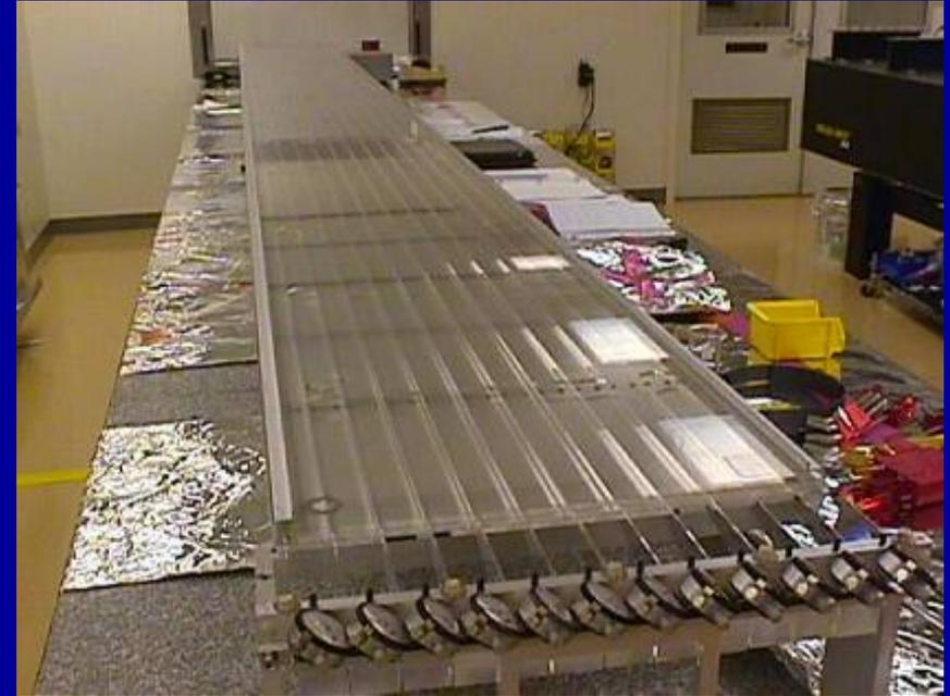
Shine HeNe laser down length of bar to verify integrity of all glue bonds
