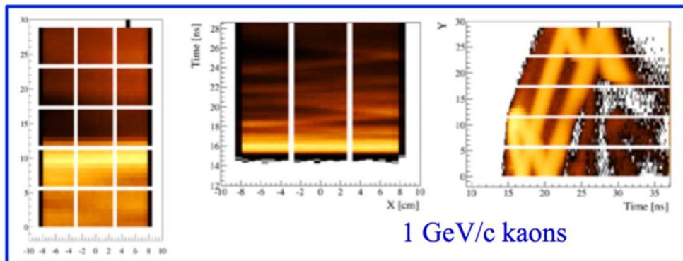
Simulation study for PANDA Barrel DIRC with wide plate geometry suggests that time-based PDFs perform significantly better than pure geometric reconstruction.
