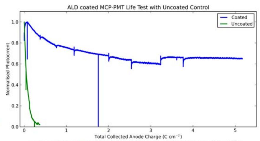
Test of relative efficiency as a function of collected anode charge. Breaks in the plot were created when the detector was taken out of the setup for other testing.
