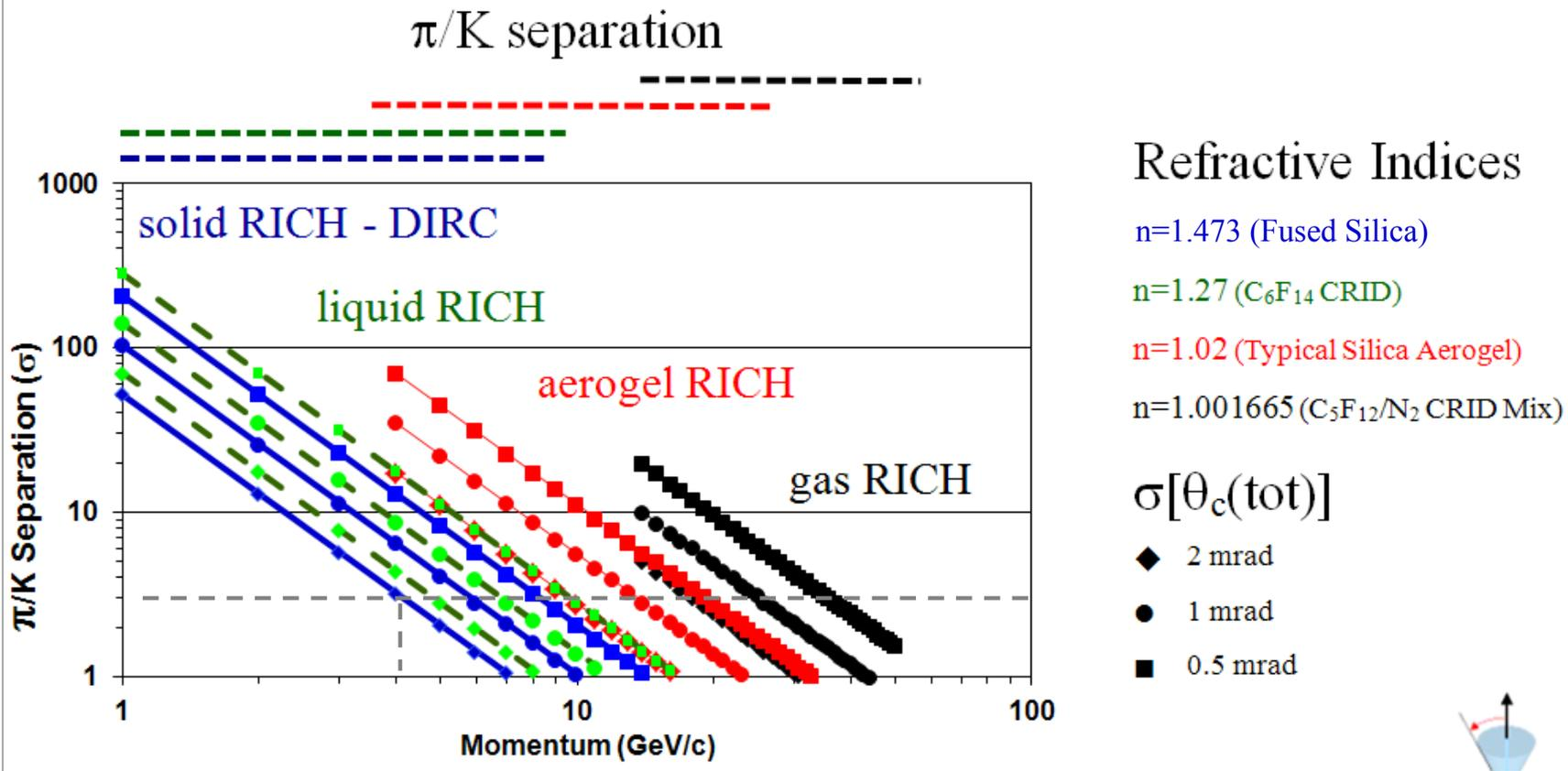
DIRC provides good  $\pi/K$  separation potential significantly beyond 4 GeV/c.
