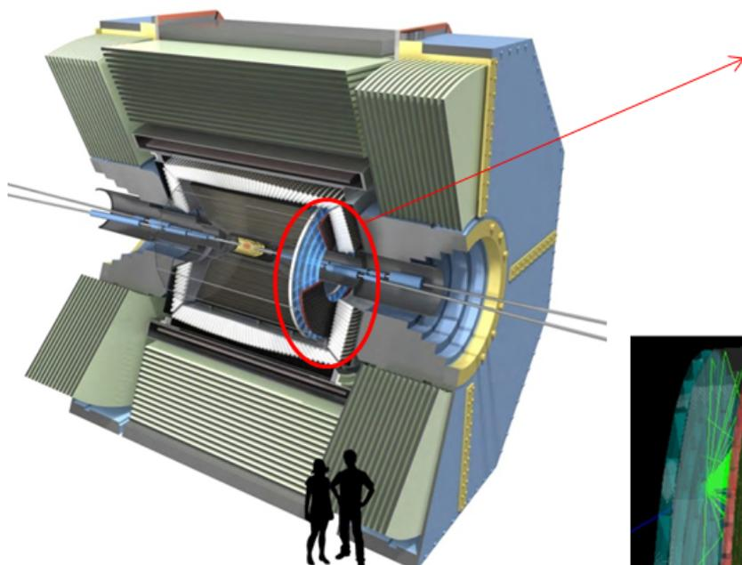
Replace threshold-type Aerogel Cherenkov Counter to **Aerogel RICH**
