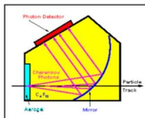
Cherenkov lights are reflected with a common mirror and are detected with 1934 phototubes of 3/4 inch diameter.
