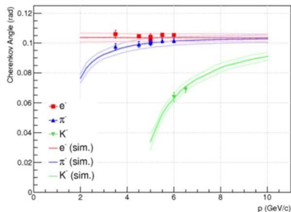
*R&D on high momentum particle identification with a pressurized Cherenkov radiator,*
