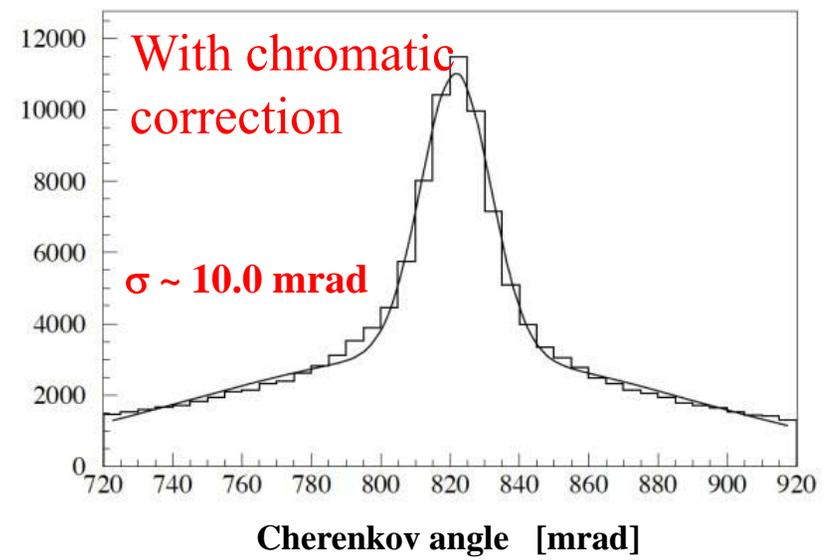
Use correlation from data to correct  $\theta_c$  by time. We gain about  $\sim 0.8$  mrad. MC expects a gain of  $\sim 1$  mrad. We hope to further improve this correction by improving timing resolution.
