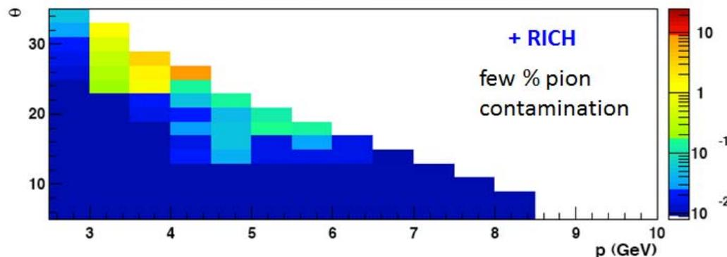
Even with a not yet optimized tuning of pattern recognition and likelihood ID, the  $\pi$  contamination is of the order of 1%
