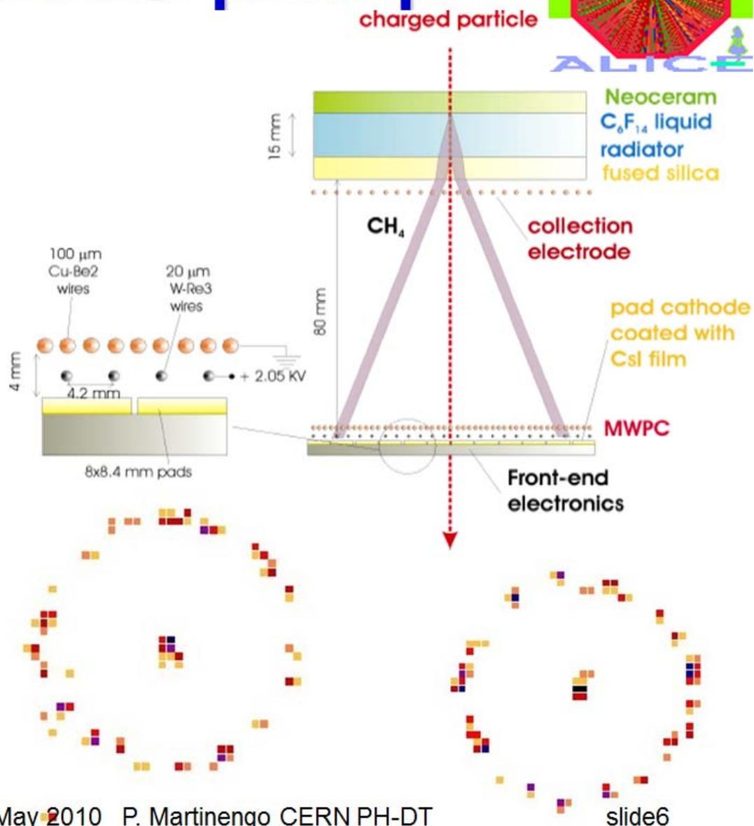
*R&D on high momentum particle identification with a pressurized Cherenkov radiator,*
