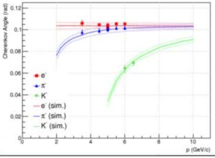
R&D on high momentum particle identification with a pressurized Cherenkov radiator, M. Weber, Mon 16:35
