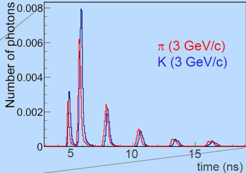
To distinguish K/ $\pi$ , the 'ring' image has to propagate undistorted along the bar and measured with good timing resolution ( $\sim 50$  ps).
