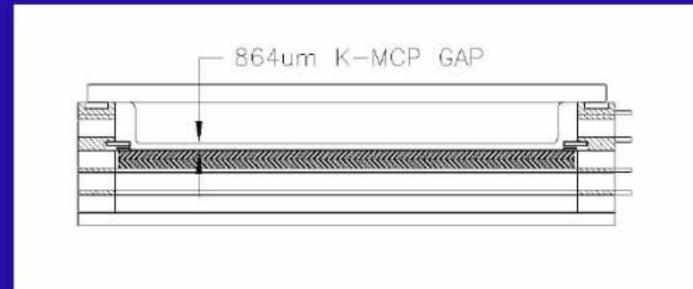
Penalty of this design: the efficiency drops to zero near edges.
