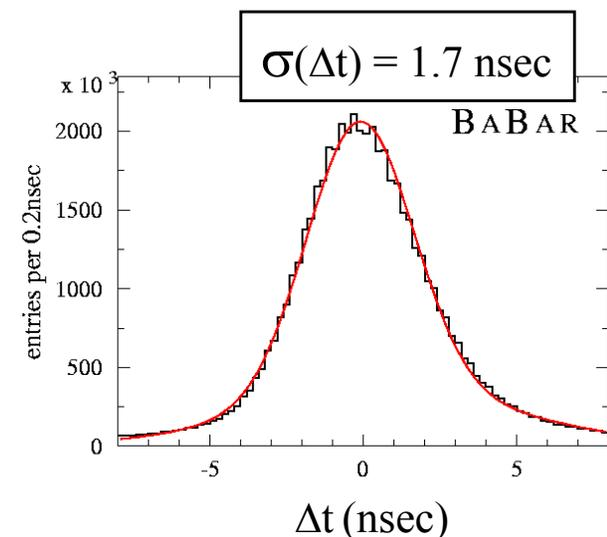
$\Delta t$  also used to determine event time for “self-triggering” of DIRC.
