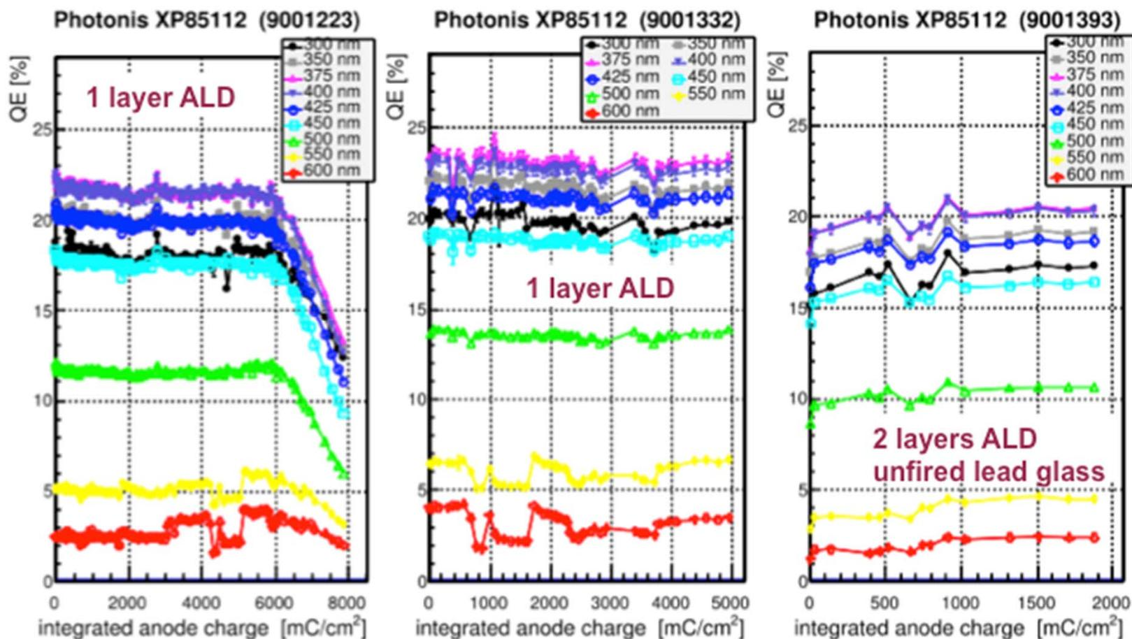
PHOTONIS Planacon with 1 layer ALD: no QE loss up to 5 C/cm<sup>2</sup>
