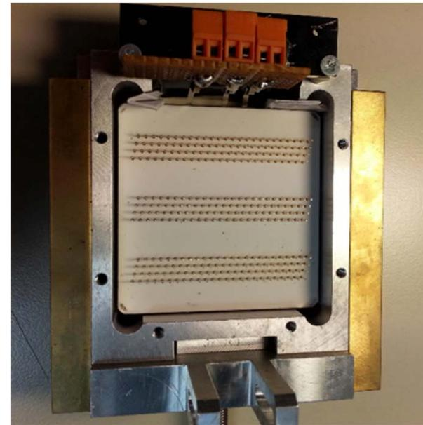
Rear view (anode pin array) in holder
