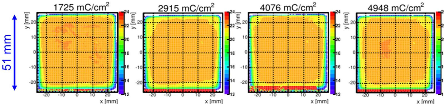
→ no visible QE degradation up to 6C/cm<sup>2</sup>, loss limited to illuminated half.
