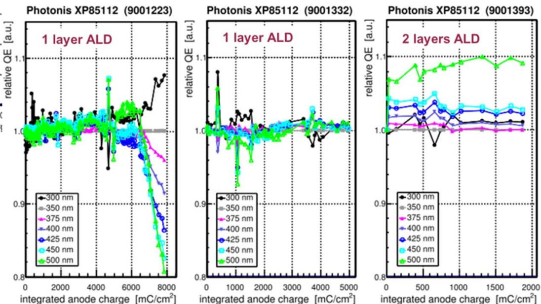
→ Clear difference in wavelength-dependent aging between different methods.
