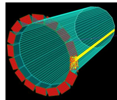
PANDA DIRCs require compact, fast multi-pixel sensor with single photon sensitivity in strong magnetic field with trigger-less DAQ and 20MHz average interaction rate.
