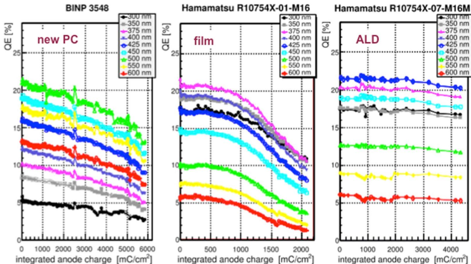
BINP new PC: continuous QE degradation
