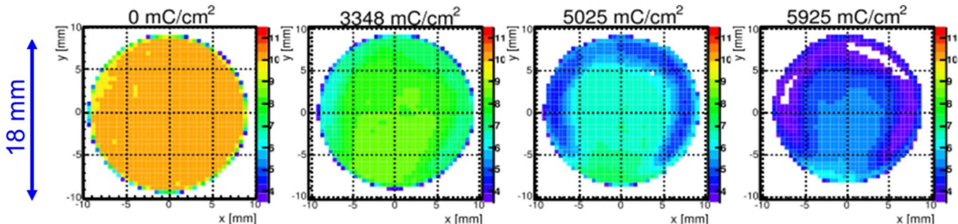
→ QE degradation evolves from rims and corners, both film and new PC fail.
