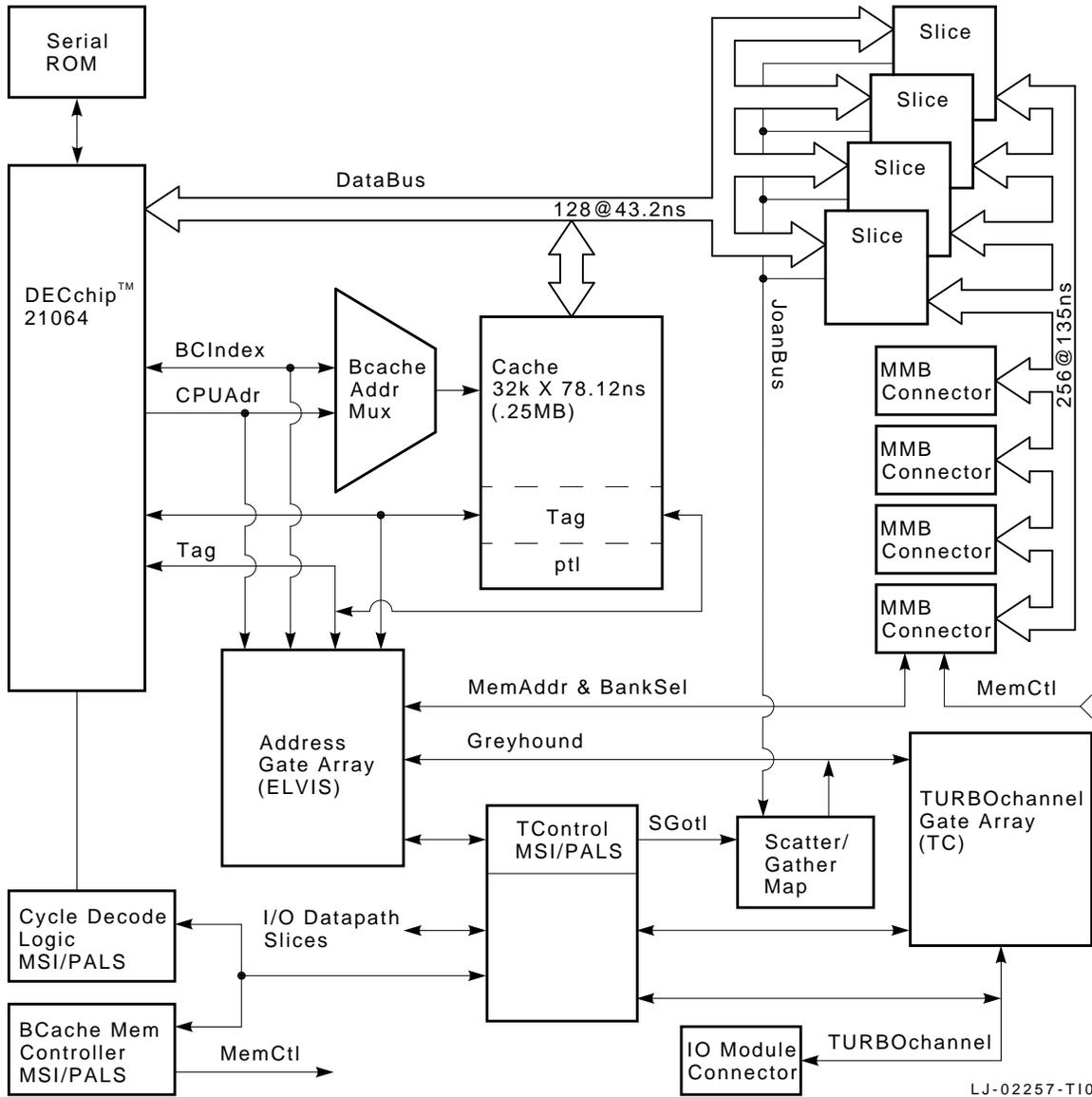
**Interconnection:** The system card (Syscard) provides connectors to interface to the DEC 3000 Model 400/400S AXP system I/O
