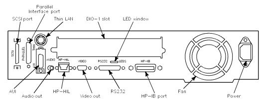
Figure 1-2. Model 382 Controller Rear Panel
