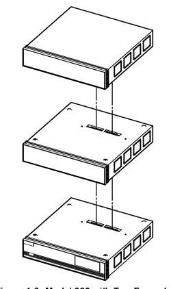
Figure 1-3. Model 382 with Two Expanders
