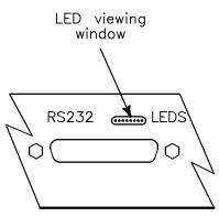
Figure 7-1. Rear Panel Viewing Slot for Diagnostic LEDs
