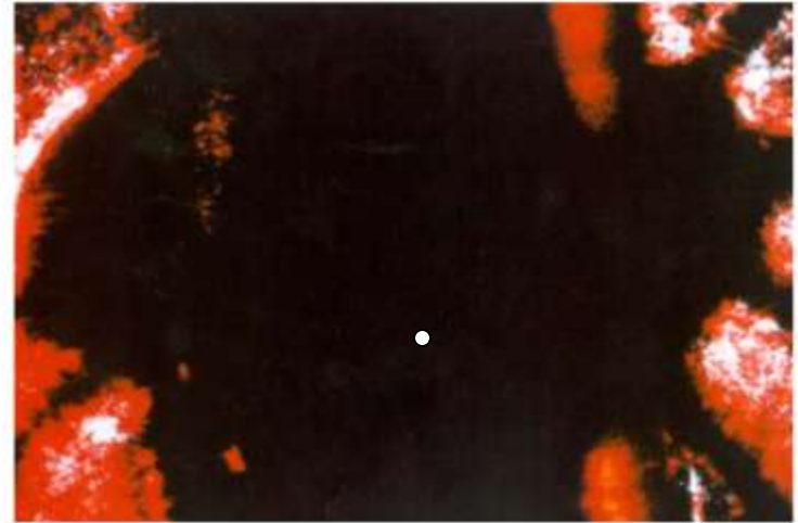
Optical Detection of a Single Barium Ion in a Paul Trap Dehmelt, Toscheck et al.
