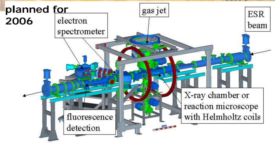
Recoil ion spectrometer:present target chamber will be replacedA longitudinal B field and ain 2006 by the recoil ion chamberwill allow to detect low morrin 2006 by the recoil ion chamberand target recoil ionsin 2006 by the recoil ion chamber
