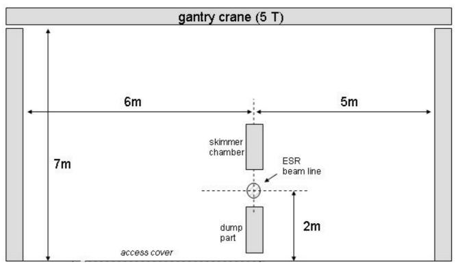
distance between beam pipe and the outer NESR concrete wall: 5 m distance between beam pipe and the inner NESR concrete wall: 6 m length of the experimental area: 19 m height experimental area: 7 m
