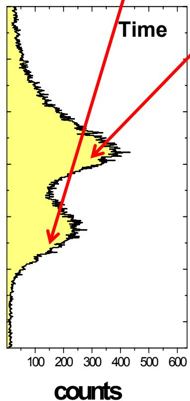
Recombination into Rydberg states leads to the delayed Lyman emission, by up to microsecond.
