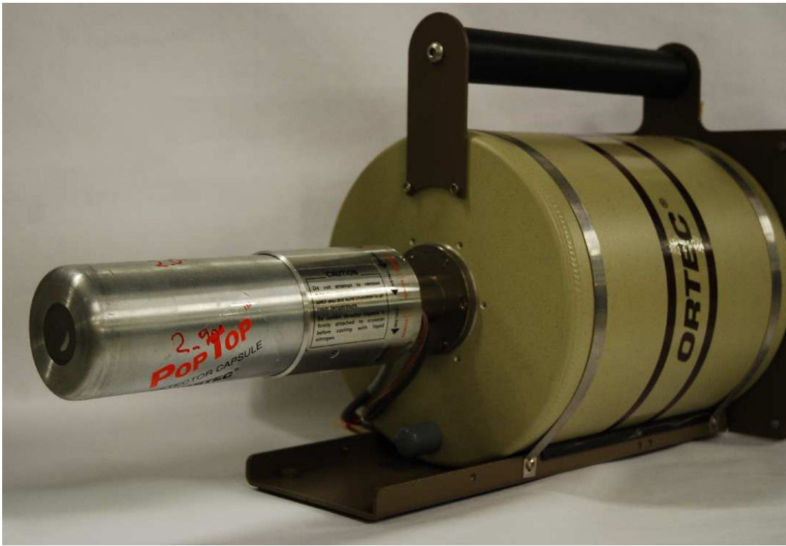
Figure 5.7: The high-purity germanium x-ray detector (ORTEC) used in the experiment.
