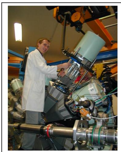
The current idea is now to use the triangular flanges to hold the detectors and enable the existing manipulator (or one very similar) to be used.
