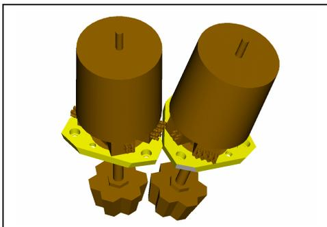
This configuration has the dummy connector box (no connectors present) adjacent to the neighbouring detector in the first ring.
