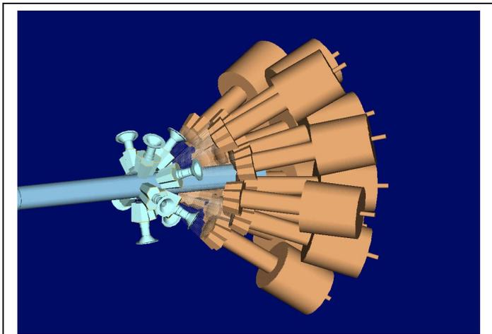
Figure 1. Schematic layout of the Cluster and Miniball detectors in the fast beam Rising configuration. A 160mm diameter beam pipe passes through the array.
