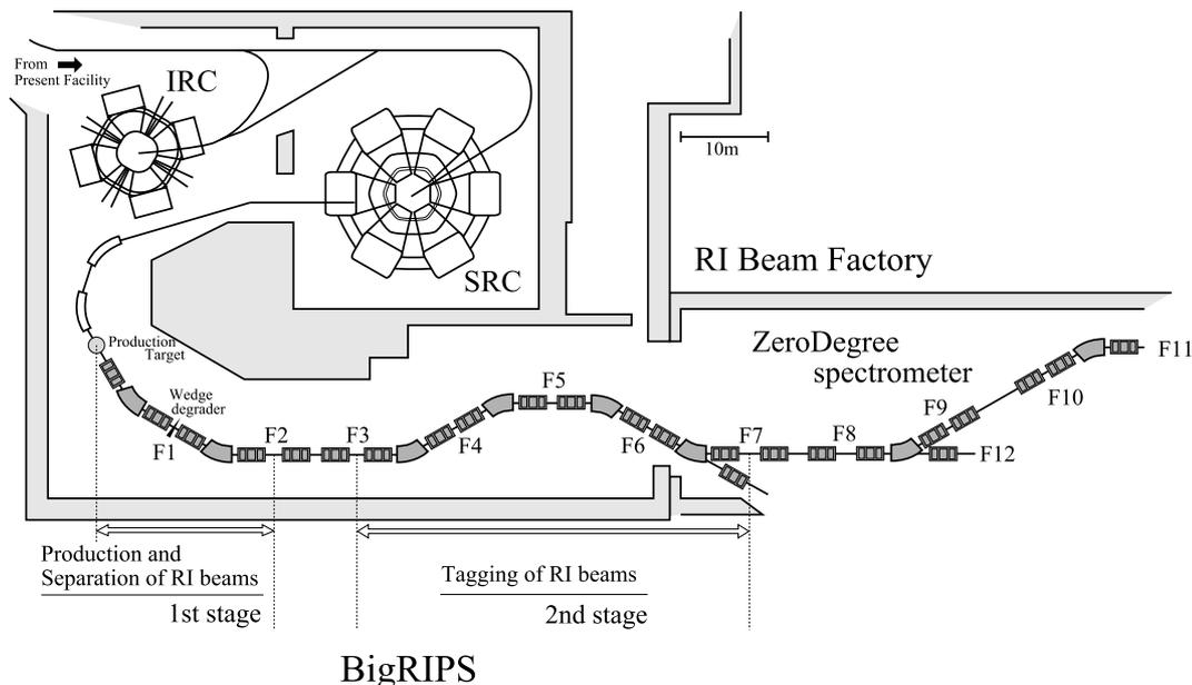
Figure 1: Overview of the RIBF facility. The radioactive ion beams are produced and separated with the BigRIPS fragment separator and transported to the focus F11, the location of the E(U)RICA spectrometer.
