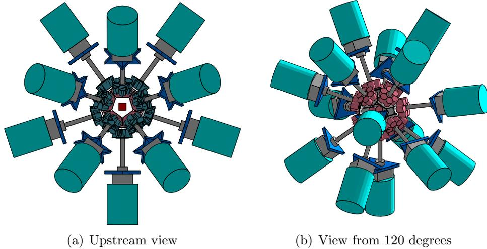
Figure 2: Schematic layout of the E(U)RICA spectrometer. The 15 Cluster detectors are arranged in three rings at angles of 51, 90, and 129 degrees, respectively, and distances of about 200 mm.
