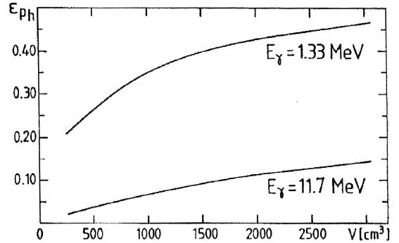
Fig. 2. Photopeak efficiency of an idealized cylindrical Ge detector of equal length and diameter as function of volume. A constant solid angle of  $\Omega = 0.0136$  is assumed.
