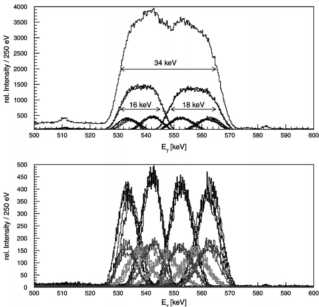
Fig. 3. Overlay of the Doppler broadened line shape of the 547.5 keV  $^{197}\text{Au}$  line (see text).
