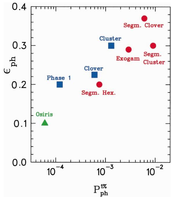
Fig. 5. Related values of intrinsic photopeak efficiency  $\epsilon_{ph}$  and maximal total photopeak efficiency  $P_{ph}^{1\%}$  for one detector, obtained under the requirement of an energy resolution of 1% for a  $\gamma$ -emitter moving with  $v/c = 10\%$  perpendicular to the detector. The triangles corresponds to a typical pre-Euroball detector, squares mark the various Euroball detector types and circles correspond to newly developed segmented Ge detectors.
