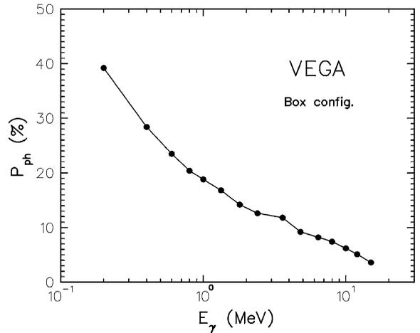
Fig. 4. Total photopeak efficiency  $P_{ph}$  as a function of the  $\gamma$ -energy for the Vega array in the compact box-like configuration.
