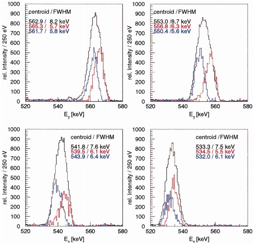
Fig. 6. 547.5 keV line of  $^{197}\text{Au}$  for four segments at different scattering angles (black) and examples for line shapes with reduced width (red, blue) obtained by choosing certain interaction positions of the  $\gamma$ -rays through pulse shape analysis.
