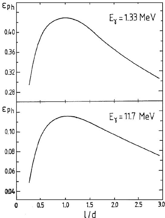
Fig. 1. Photopeak efficiency as function of the ratio between length and diameter  $l/d$  of an idealized cylindrical Ge detector. A volume of  $2000 \text{ cm}^3$  was assumed, approximately matching the total active volume of the Super Segmented Clover detector. The simulation calculations using the code GEANT3 [8] are based on a constant solid angle of  $\Omega = 0.0136$ .
