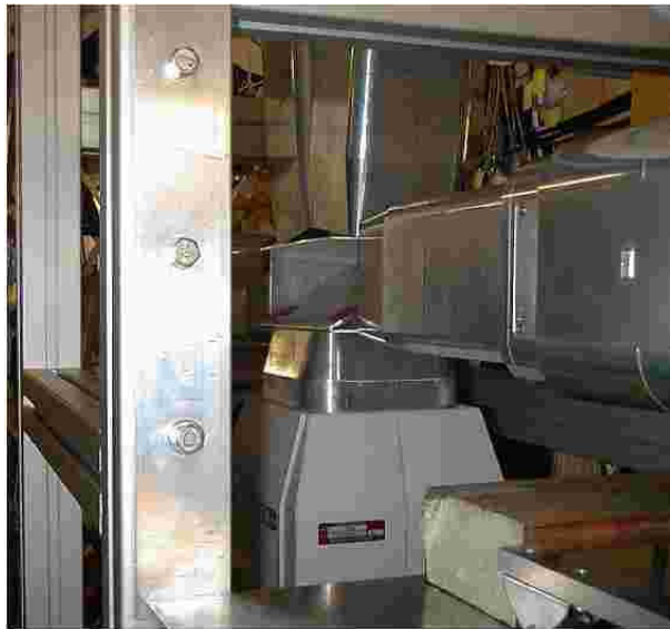
Figure 3.7: Photo of the final focal plane of the separator. The aluminum Z-shaped catcher of thickness 4-6 mm is surrounded by Ge clover detectors.
