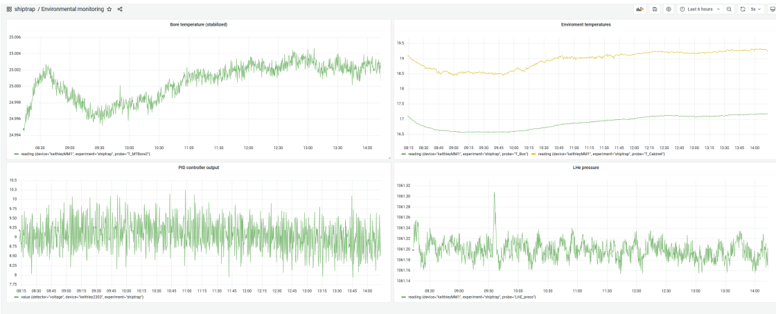
Fig. 6: Realtime visualisation of the TT , PID output voltage, environmental temperatures and the liquid helium pressure over a 6hr period using Grafana.
