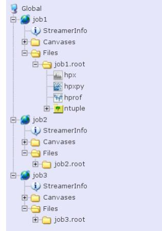
Fig.4: Tree-view display of the hierarchy elements available in a DABC application. Here several ROOT jobs are connected, files with trees can be browsed, and histograms can be displayed.
