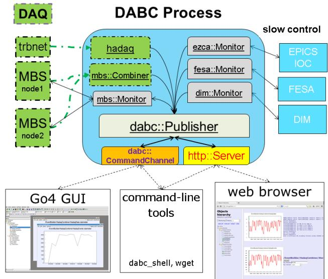
Fig.5: Schematic view of a DABC process publishing monitoring data of several plug-in sources. In addition to various slow control systems, the parameters of external MBS DAQ systems and internal DABC DAQ plug-ins may be monitored. The central *dabc::Publisher* will deliver the monitoring data both to an http server, and to a proprietary command channel socket. Here the variables of interest can be inspected with a web browser, a regular Go4 GUI, or by means of simple command-line tools, resp.
