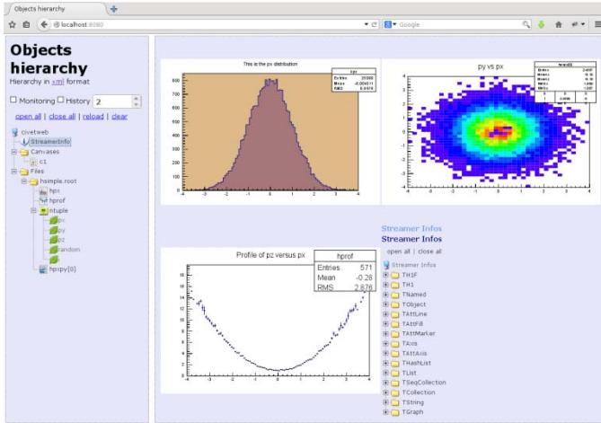
Fig.3: Browser with objects available from *hsimple.C* macro. The objects' hierarchy is on the left side, and several displayed histograms are on the right. Also a list of streamer-infos is displayed.
