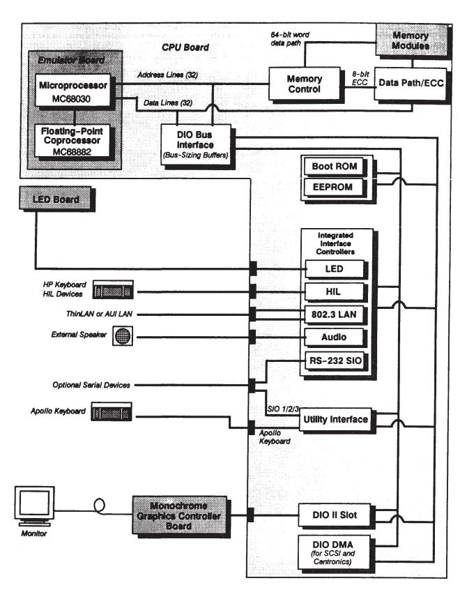
Figure 3-2. Model 400dl System Block Diagram
