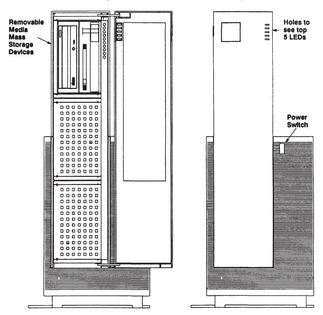
Figure 2-3. Model 400s System Unit Operational Controls
