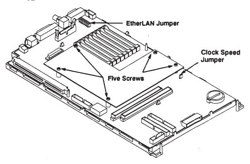
Figure 5-12. CPU Board Component Locations (Model 400t and 400dl)
