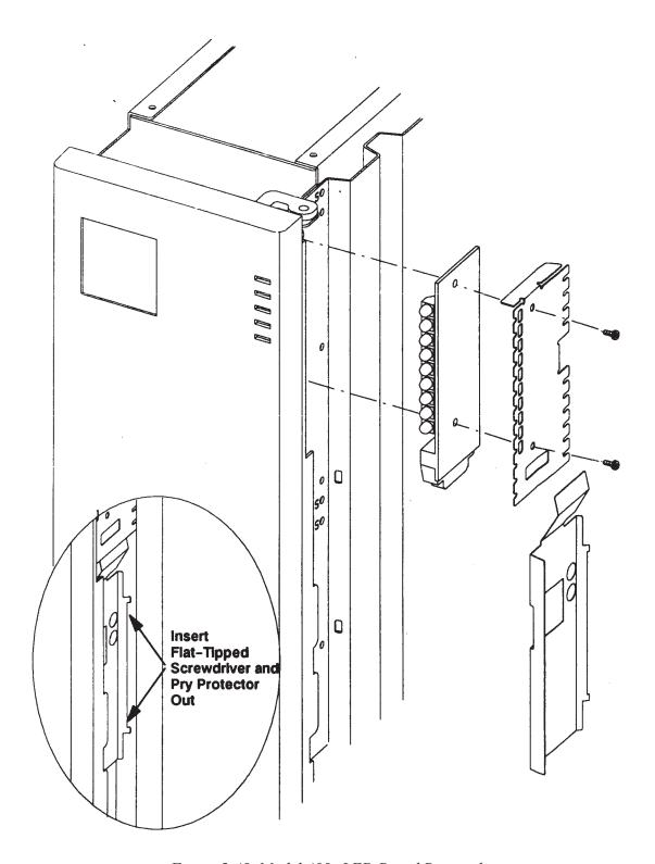
Figure 5-49. Model 400s LED Board Removal
