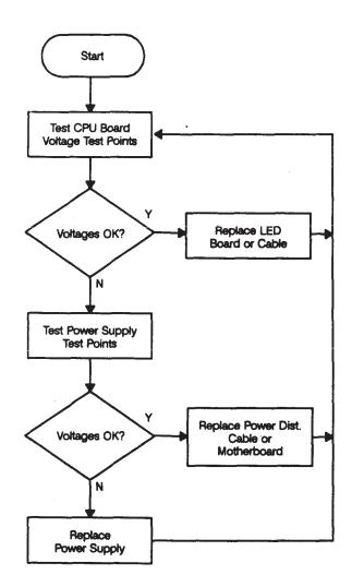
Figure 4-3. Model 400s System Power LED Not On
