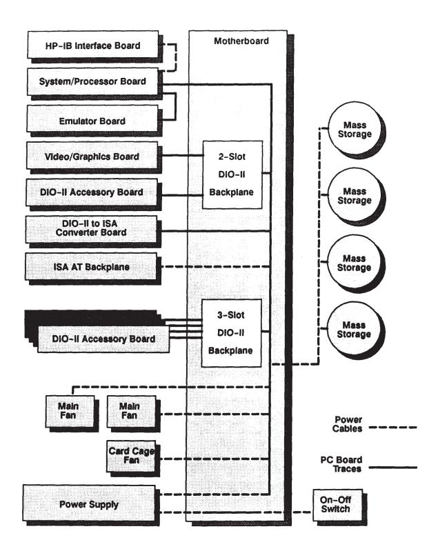
Figure 3-6. Model 400s System Unit Power Distribution Diagram
