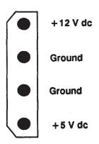
Figure 4-25. Model 400s System Unit Motherboard Mass Storage Power Distribution Connector
