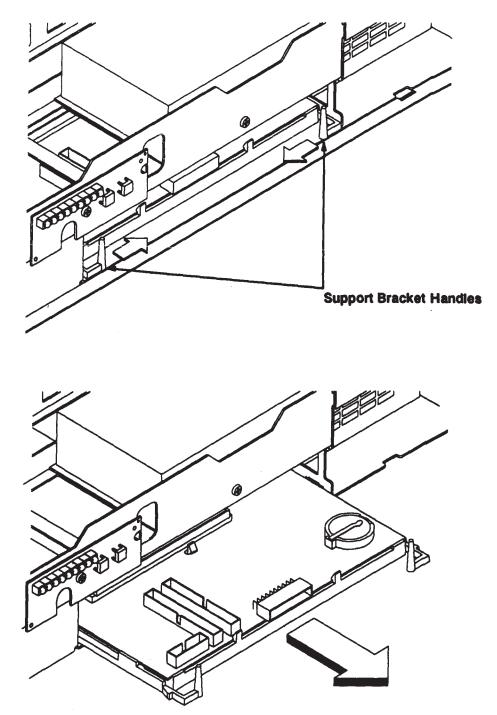
Figure 5-11. Sliding the CPU Board out of the System Unit (Model 400t and 400dl)
