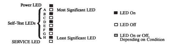
Figure 4-15. Sample Boot ROM Self-Test LEDs with Key
