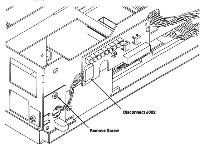
Figure 5-16. Power Switch Panel Removal (Model 400t and 400dl)
