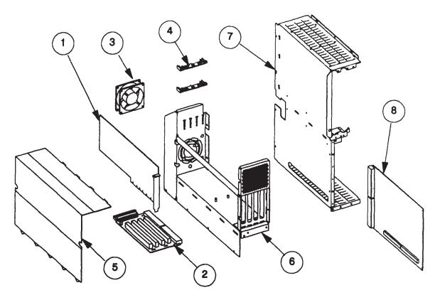
Figure 5-52. Model 400s ISA Card Cage Illustrated Parts Breakdown
