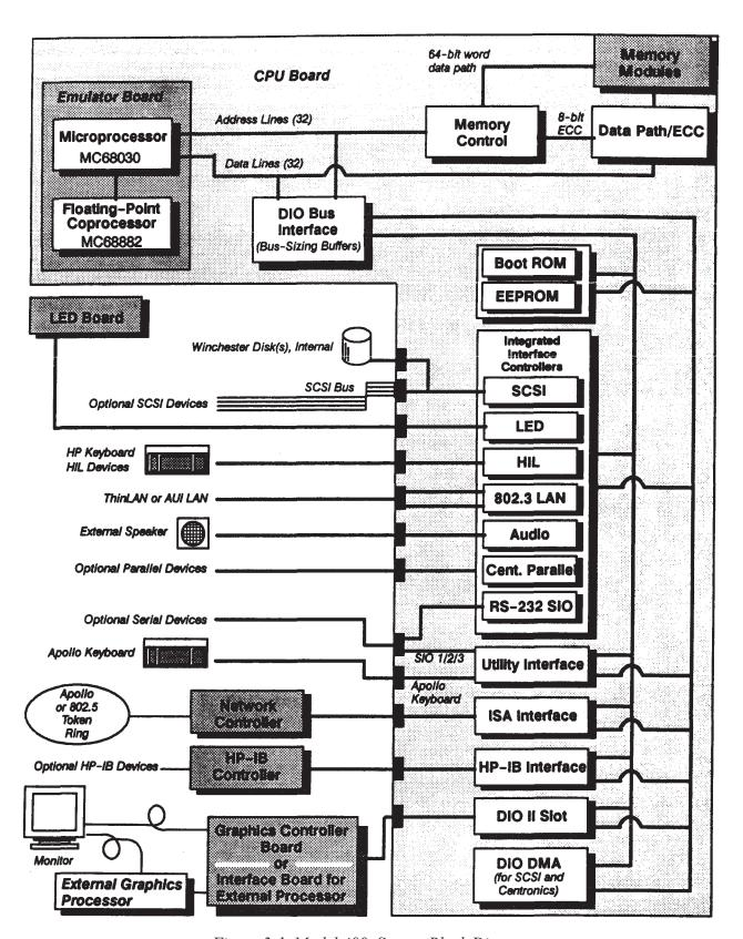
Figure 3-1. Model 400t System Block Diagram
