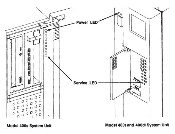
Figure 2-8. System Unit Front Panel LEDs
