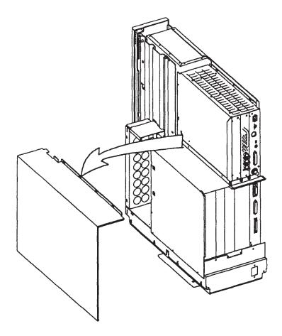
Figure 5-24. Model 400s Right Side Cover Removal
