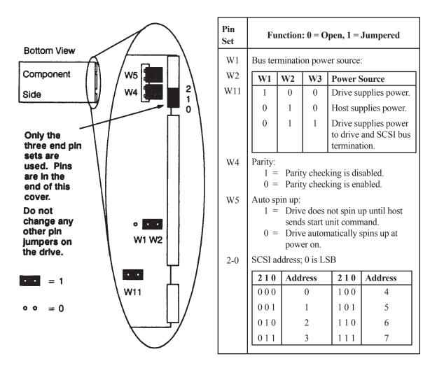
Figure A-11. HP A1444A 660 MB Micropolis Hard Disk Drive
