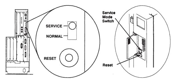
Figure C-1. System Unit Service/Normal Switch and Reset Button
