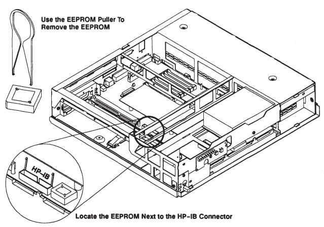
Figure 5-14. Removing the EEPROM from the System Unit (Model 400t and 400dl)
