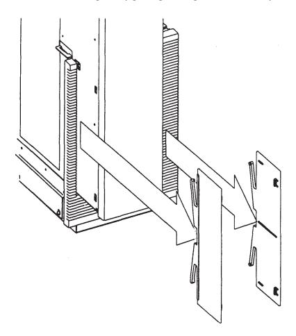
Figure 5-25. Model 400s Trim Plate Removal
