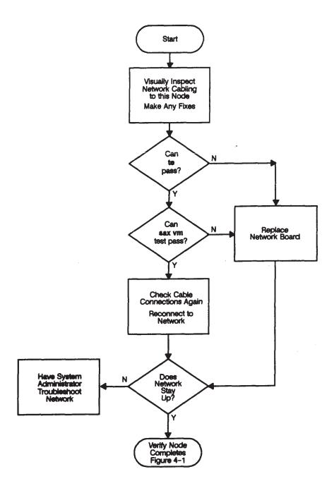
Figure 4-9. Node Causes Network Problems
