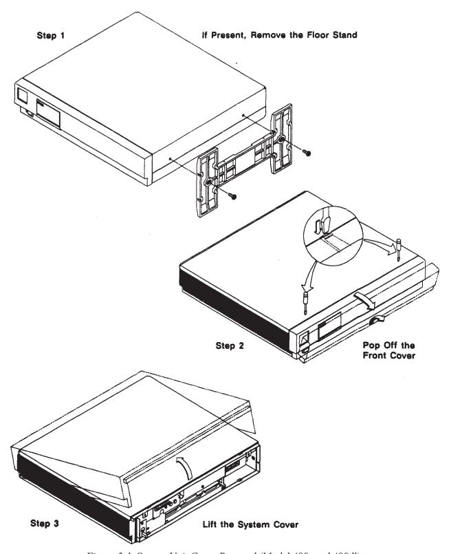
Figure 5-1. System Unit Cover Removal (Model 400t and 400dl)
