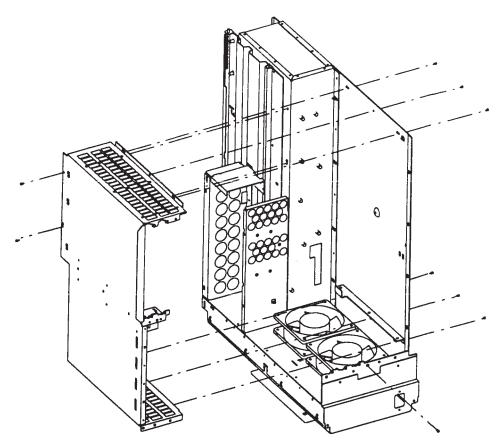
Figure 5-46. Model 400s DIO-II Center Wall Removal
