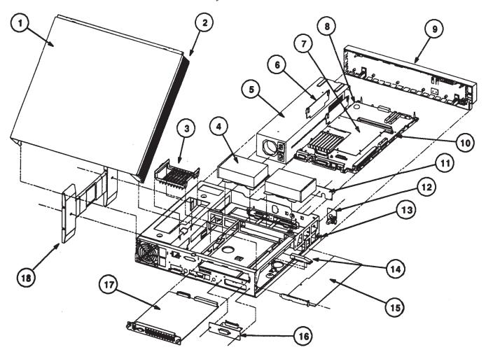
Figure 5-20. Illustrated Parts Breakdown of the System Unit
