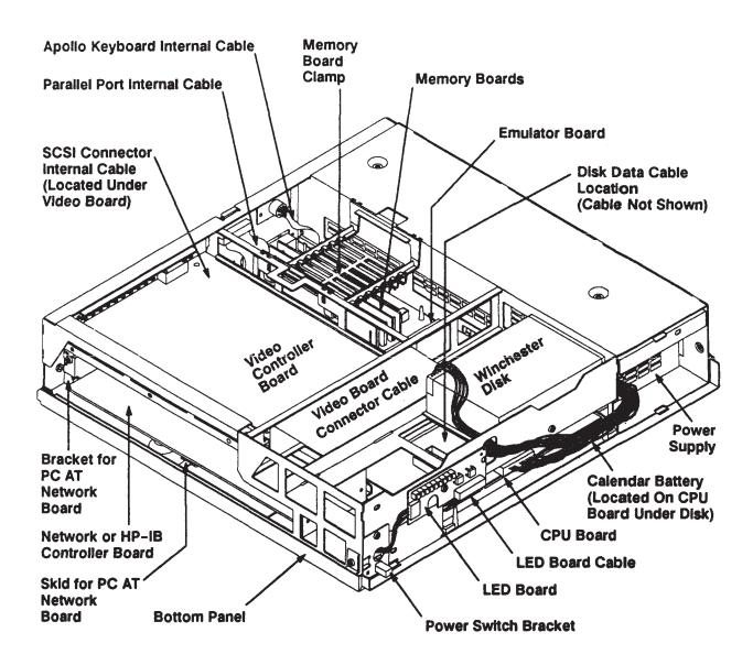
Figure 5-2. System Components (Model 400t and 400dl)
