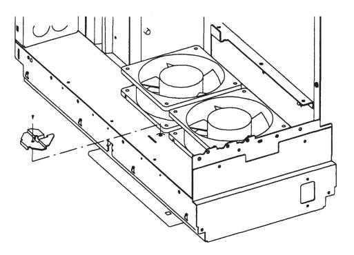
Figure 5-48. Model 400s Main Fans Removal
