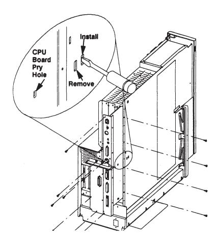
Figure 5-38. Model 400s CPU Board Removal
