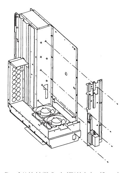
Figure 5-44. Model 400s Standard/ISA Motherboard Removal
