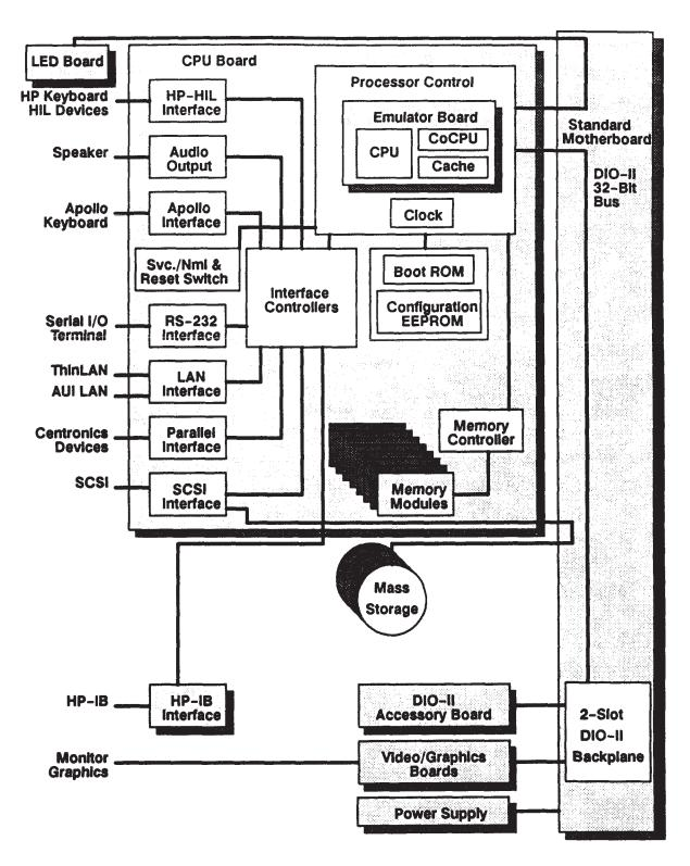
Figure 3-3. Model 400s Standard I/O System Unit Functional Block Diagram
