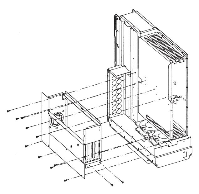
Figure 5-35. Model 400s ISA Card Cage Removal
