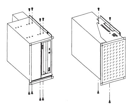
Figure 5-29. Model 400s Mass Storage Device Bracket Removal
