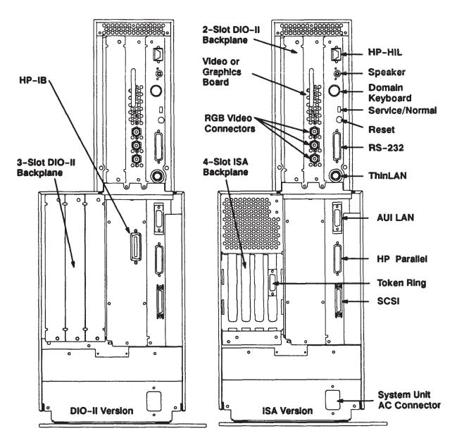
Figure 2-4. Model 400 System Unit System Connectors
