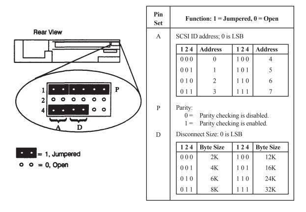
Figure A-12. HP A1449A 0.25-in. QIC 60 MB Tape Drive
