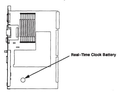
Figure 5-42. Model 400s Real-Time Clock Battery Removal
