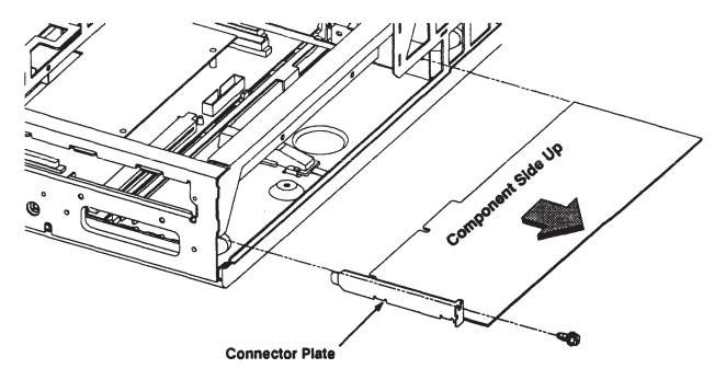
Figure 5-6. Network Interface Board Removal (Model 400t and 400dl)
