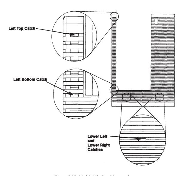
Figure 5-27. Model 400s Bezel Removal
