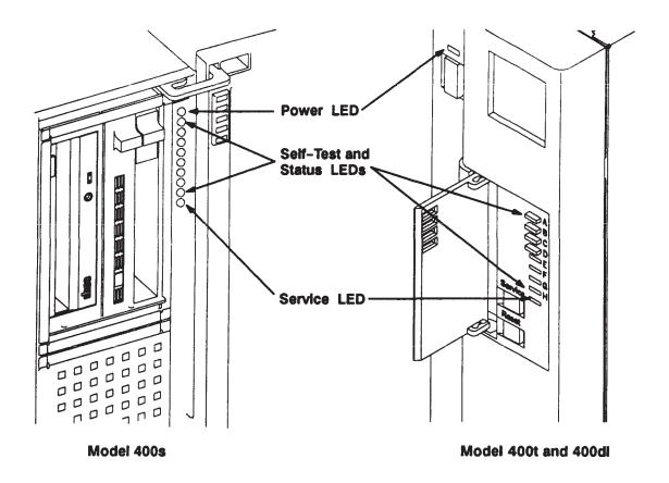
Figure 4-11. Front Panel LEDs
