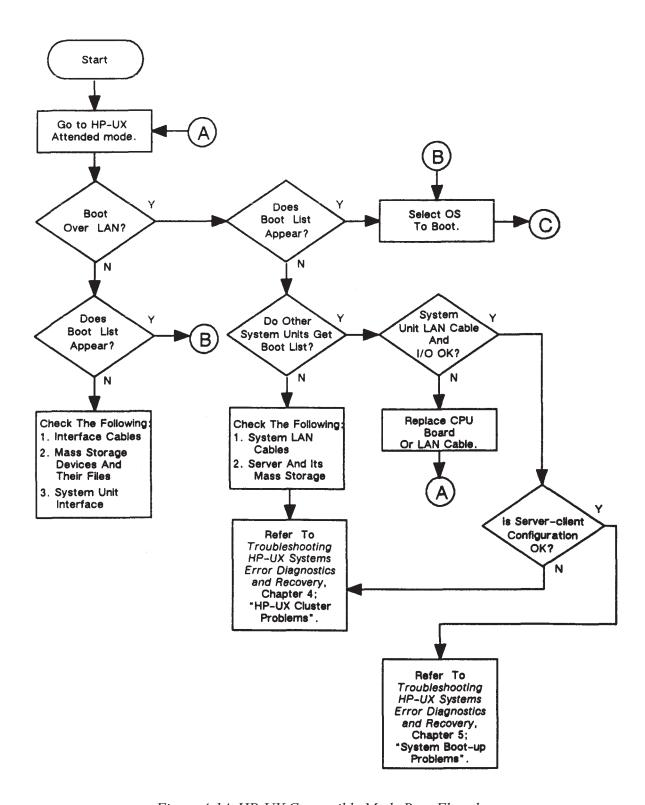
Figure 4-14. HP-UX Compatible Mode Boot Flowchart
