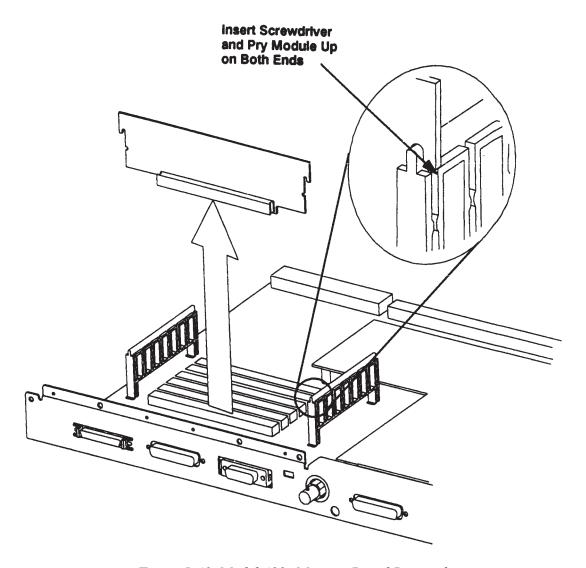
Figure 5-40. Model 400s Memory Board Removal
