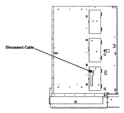
Figure 5-31. Model 400s Mass Storage Power Distribution Cable Removal
