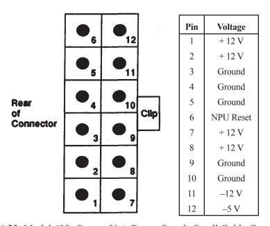
Figure 4-23. Model 400s System Unit Power Supply Small Cable Connector
