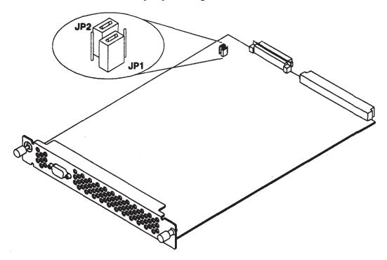
Figure A-3. VRX Monochrome Graphics Controller Jumpers
