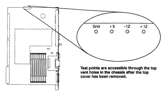
Figure 4-21. Model 400s System Unit CPU Board Voltage Test Points
