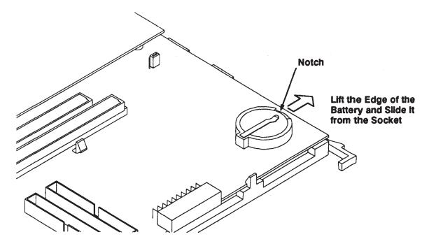
Figure 5-18. Calendar Battery Removal (Model 400t and 400dl)
