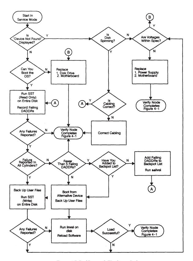
Figure 4-7. Problems with Winchester Disk
