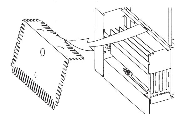
Figure 5-32. Model 400s RFI Cover Removal
