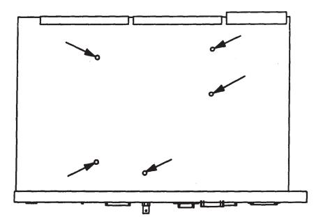
Figure 5-41. Model 400s Emulator Board Screws
