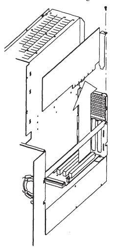
Figure 5-33. Model 400s ISA Board Removal
