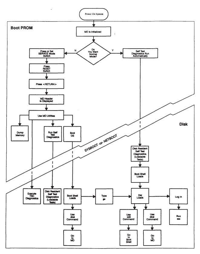
Figure 4-10. Diagnostic Relationships for Domain/OS Compatible Mode
