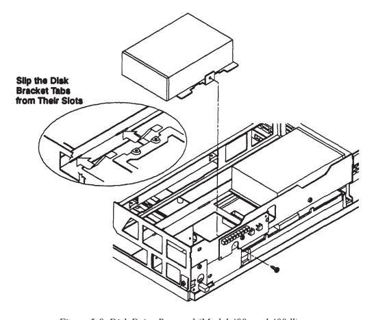
Figure 5-8. Disk Drive Removal (Model 400t and 400dl)
