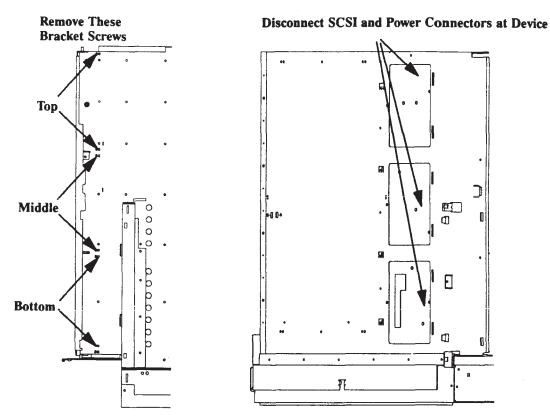
Figure 5-28. Model 400s Mass Storage Device Removal
