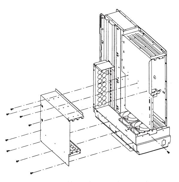
Figure 5-45. Model 400s 3-Slot DIO-II Card Cage Removal
