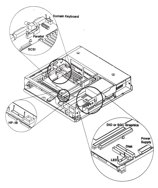
Figure 5-10. Disconnecting Internal Cables from the CPU Board (Model 400t and 400dl)
