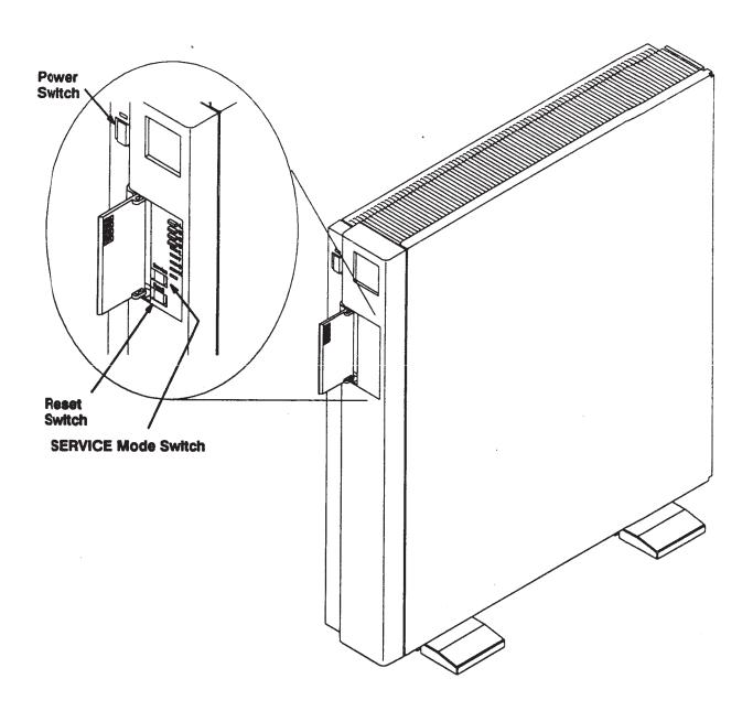
Figure 2-1. Model 400t and 400dl System
