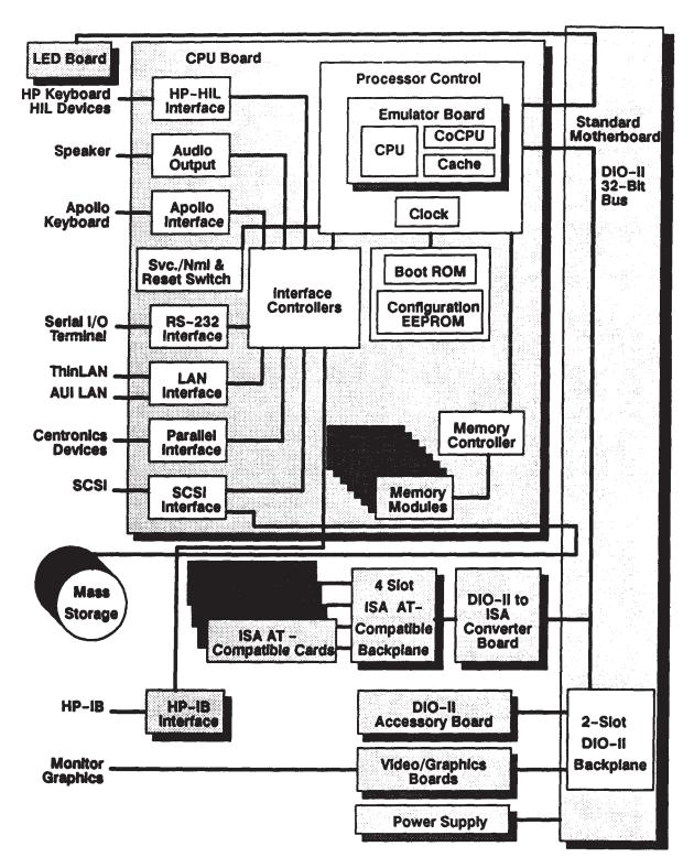
Figure 3-5. Model 400s ISA System Unit Functional Block Diagram
