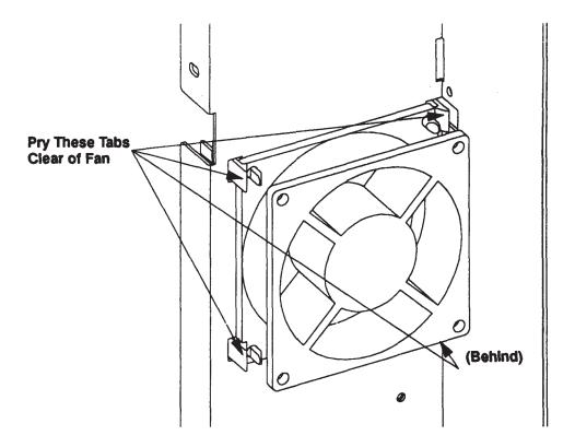
Figure 5-36. Model 400s Card Cage Fan Removal
