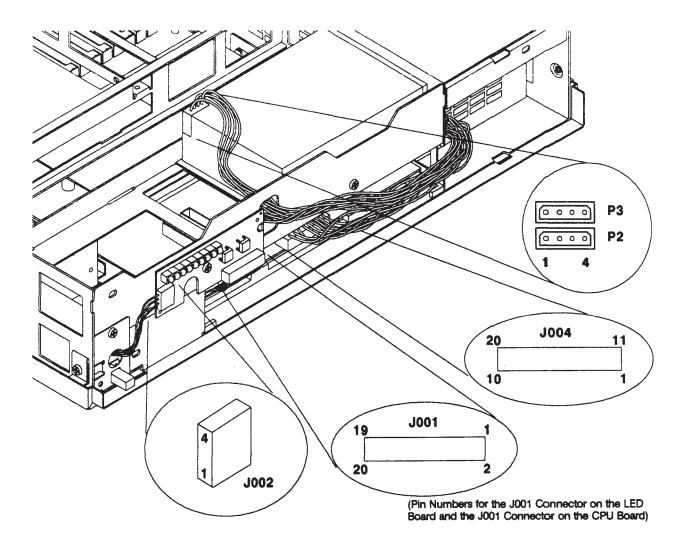
Figure 4-18. Power Connections (Model 400t and Model 400dl)
