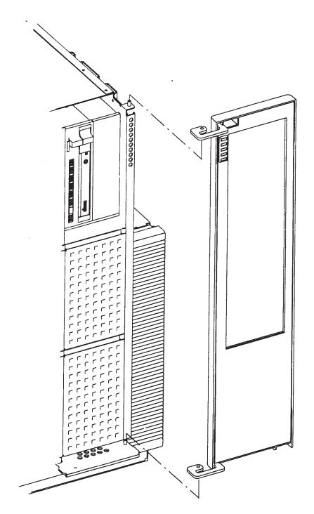
Figure 5-26. Model 400s Front Door Removal
