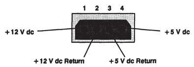
Figure 4-19. Disk Drive Power Supply Input Connector (P2 or P3)
