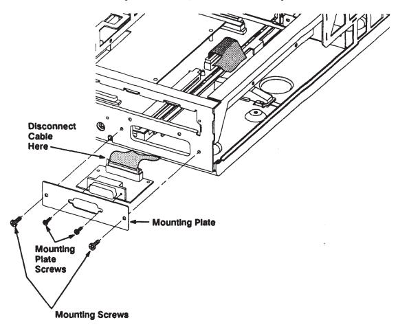
Figure 5-7. HP-IB Interface Board Removal (Model 400t and 400dl)
