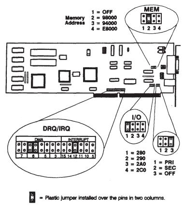
Figure A-4. Standard 802.5 Network Controller-AT Jumper Configuration
