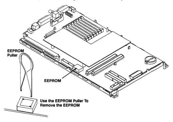
Figure 5-13. Removing the EEPROM (Model 400t and 400dl)
