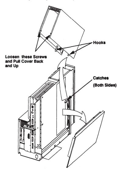
Figure 5-23. Model 400s Top and Left Side Cover Removal
