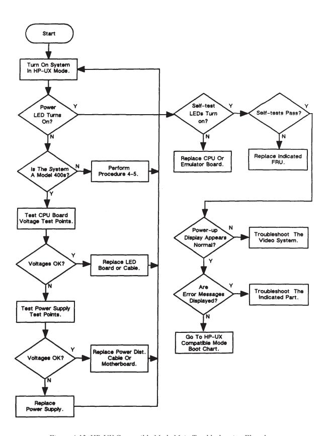
Figure 4-13. HP-UX Compatible Mode Main Troubleshooting Flowchart
