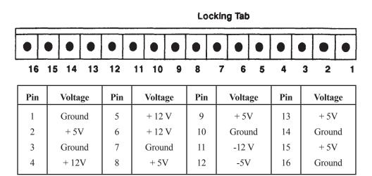
Figure 4-24. Model 400s System Unit ISA Backplane Power Cable Connector
