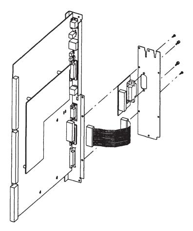
Figure 5-37. Model 400s HP-IB Board Removal
