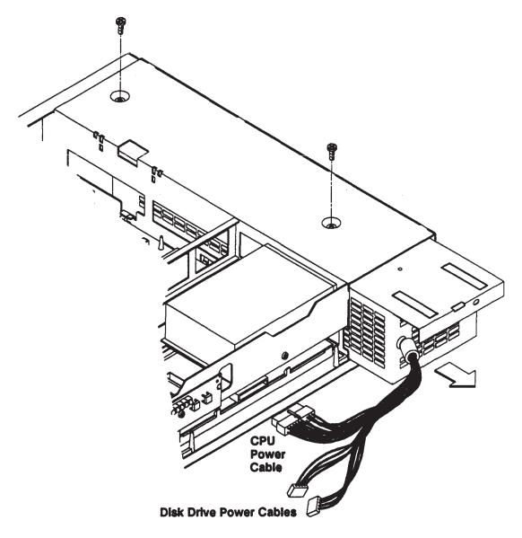
Figure 5-15. Power Supply Removal (Model 400t and 400dl)
