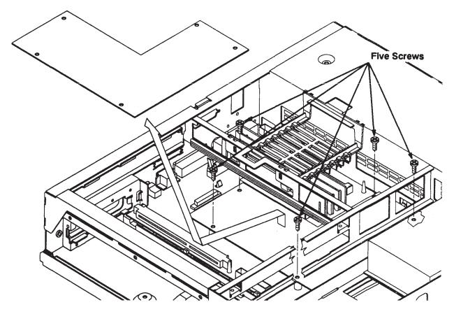
Figure 5-9. Emulator Board Removal (Model 400t and 400dl)
