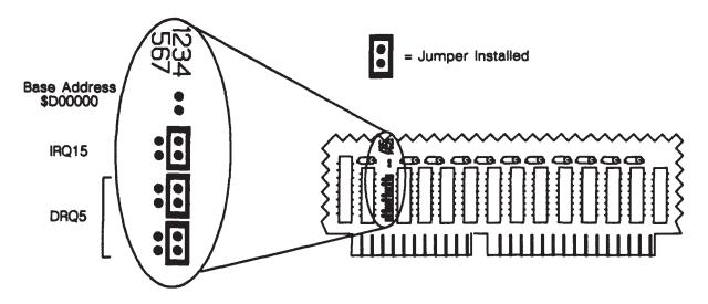
Figure A-8. PC Coprocessor Alternate Jumper Configurations
