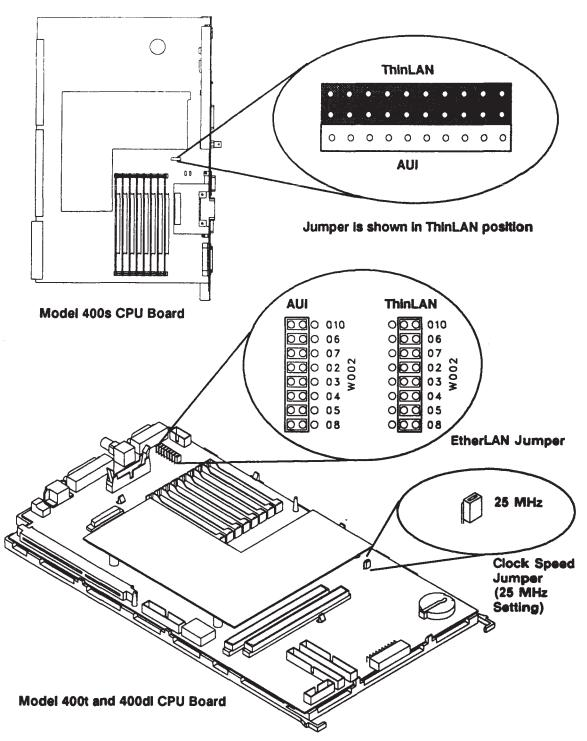
Figure A-1. CPU Board Configurations
