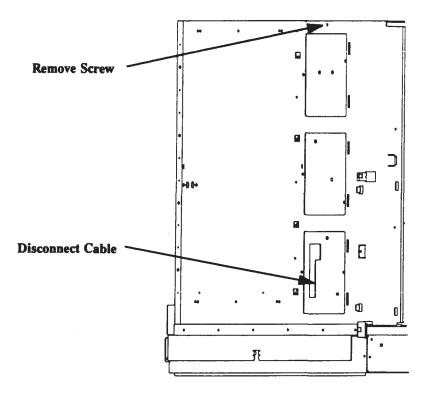
Figure 5-30. Model 400s Internal SCSI Cable Removal
