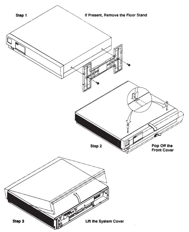
Figure 4-17. System Unit Cover Removal (Model 400t and Model 400dl)
