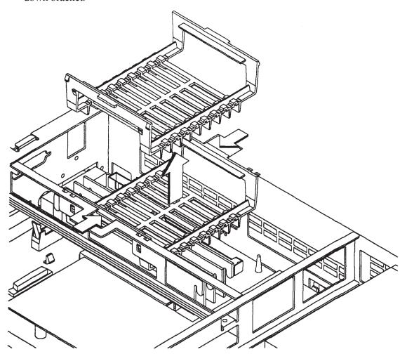
Figure 5-4. Memory Board Removal (Model 400t and 400dl)
