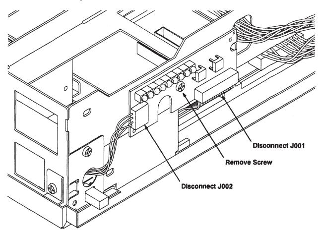
Figure 5-17. LED Board Removal (Model 400t and 400dl)
