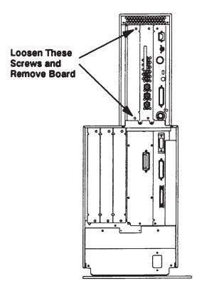
Figure 5-21. Model 400s DIO-II Accessory Board Removal
