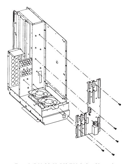
Figure 5-47. Model 400s DIO-II Motherboard Removal
