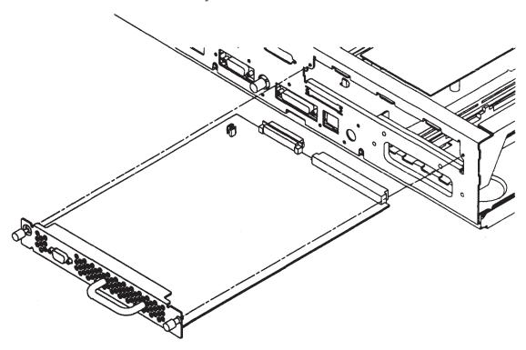
Figure 5-5. Graphics Controller Removal (Model 400t and 400dl)
