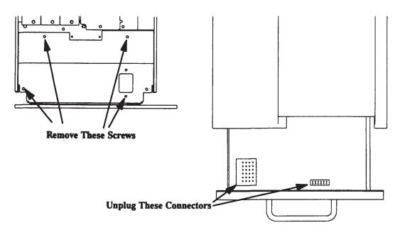
Figure 5-22. Model 400s Power Supply Removal
