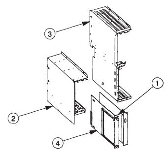
Figure 5-51. Model 400s DIO-II Card Cage Illustrated Parts Breakdown
