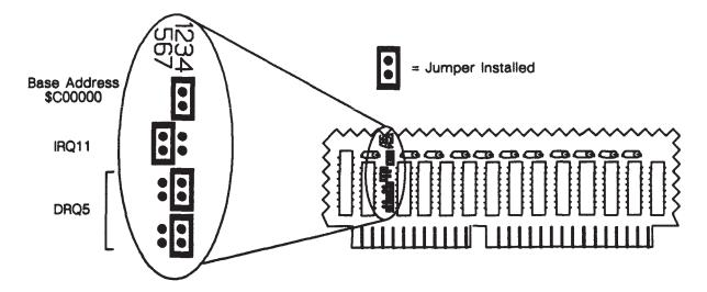
Figure A-7. PC Coprocessor Standard Jumper Configurations
