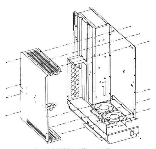
Figure 5-43. Model 400s ISA Center Wall Removal
