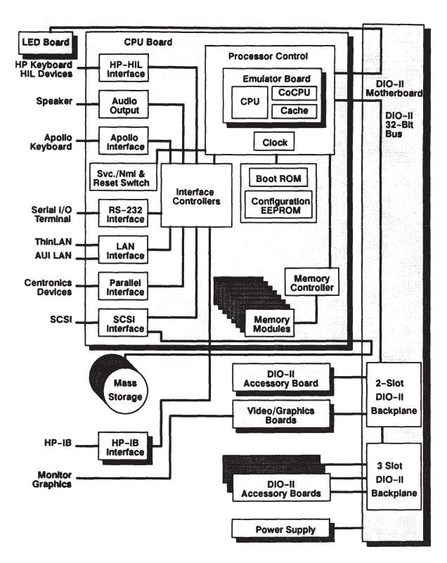
Figure 3-4. Model 400s DIO-II System Unit Functional Block Diagram
