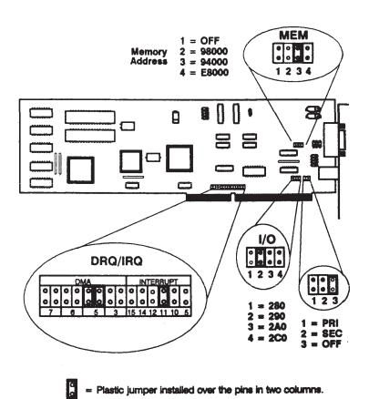
Figure A-5. Alternate 802.5 Network Controller-AT Jumper Configuration
