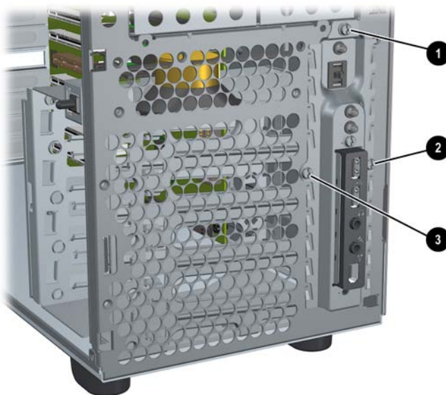
Unscrewing the front control module
