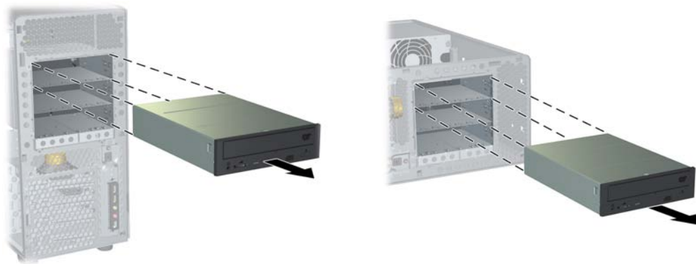
Removing an optical drive from tower and rack-mounted systems
