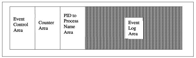
Figure 8. Shared-Memory Buffer Structure
