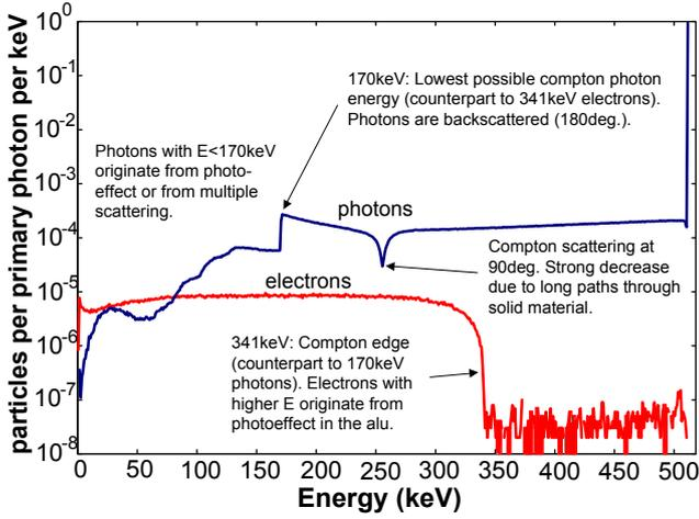
Fig. 2. Particle currents in the 0.2 mm layer of the gas gap.
