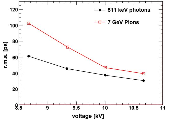
Fig. 6. Simulated time resolution as a function of the applied HV for photons and particles. For particles the simulations confirm the measurements while for photons the simulated results show a timing resolution that is much better than measured results. Moreover, the simulated time resolution improves when increasing the HV, while the measured results are essentially independent from the applied HV.
