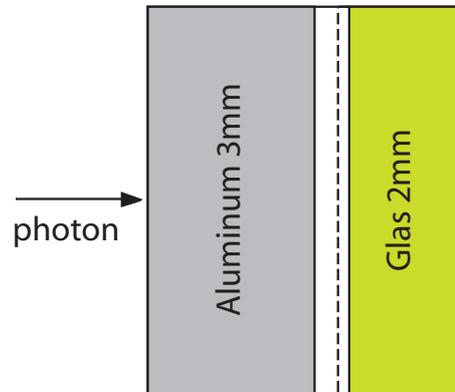
Fig. 1. RPC geometry investigated in this publication. It is similar to the one described in Ref. [3]. The photon enters either through the metal or glass electrode. For our analysis we divide the gas gap in two layers of 0.2 mm and 0.1 mm, respectively. The gas mixture is  $\text{C}_2\text{F}_4\text{H}_2$  (96.7 %) /  $\text{i-C}_4\text{H}_{10}$  (3 %) /  $\text{SF}_6$  (0.3 %).
