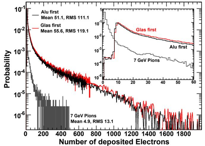
Fig. 4. Number of Electrons produced in the 0.2 mm layer of the gas gap for 511 keV photon interactions from both sides of the detector (aluminium first or glass first) and for 7 GeV pions. For the pions the mean free path between interactions is 0.1 mm and each interaction produces a fluctuating number of electrons. The insert shows in more detail the region with small electron numbers.
