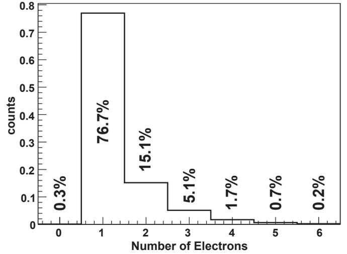
Fig. 3. Distribution of the number of electrons entering the 0.2 mm layer of the gas gap. In 76.7% of the cases there is just a Compton electron. 23% of the events are more complex.
