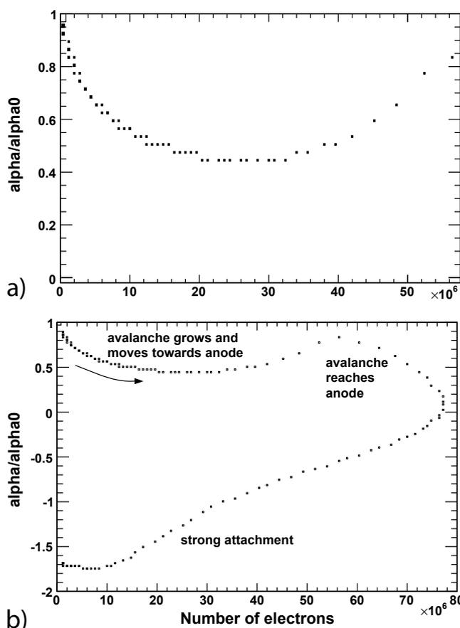
Fig. 8. Simulated evolution of the average effective Townsend coefficient  $\alpha_{eff}$ . We scale with the initial effective Townsend coefficient at the applied electric field ( $\alpha_0$ ). It is worth pointing out that the pattern visible in the upper panel is the same as found in a previous measurement (Fig. 6 in Ref. [13]).
