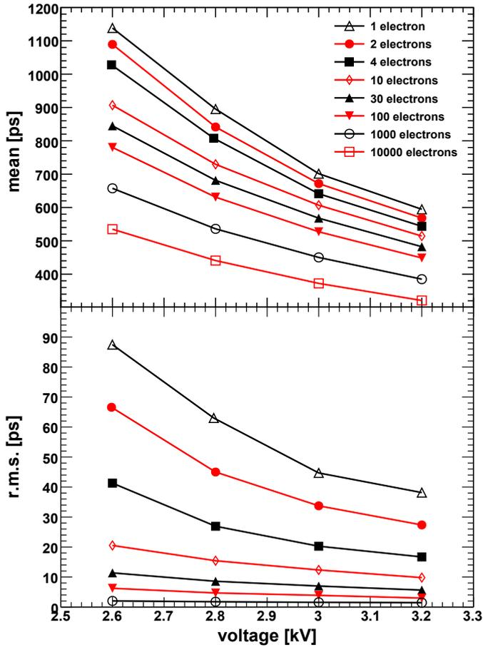
Fig. 5. Mean threshold crossing time (top) and r.m.s. (bottom) for avalanches started by a different number of electrons as a function of the applied HV. By increasing the HV for a fixed electron number the threshold crossing time is shifted to earlier times and the fluctuations around that value decrease. A larger charge for a fixed high voltage leads to earlier threshold crossing and smaller fluctuations as well.
