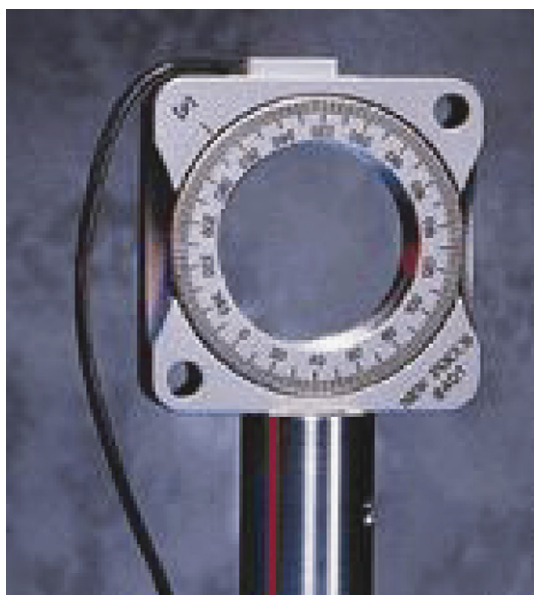
Fig. 7. Remotely controlled rotary stage [12]. The driving mechanism is based on the piezoelectric effect.
