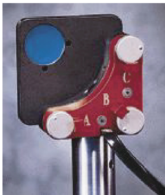
Fig. 9. Remotely controlled mirror holder [13]. The three actuators can be rotated manually or by applying series of asymmetric pulses which are converted to mechanical motion via the piezoelectric effect.
