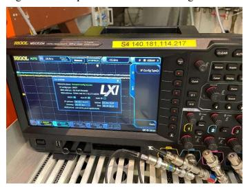
Type the numerical IP adress – 140.181.114.217 in the browser bar to connect remotely to Rigol at S4. Choose "Web Control" on the left side of the panel as shown.
