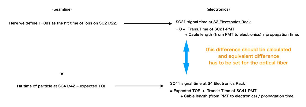
Note that RG58 (normal BNC), RG174 (normal lemo) cables have 5ns/meter, while LMR240 has 4ns/meter.
