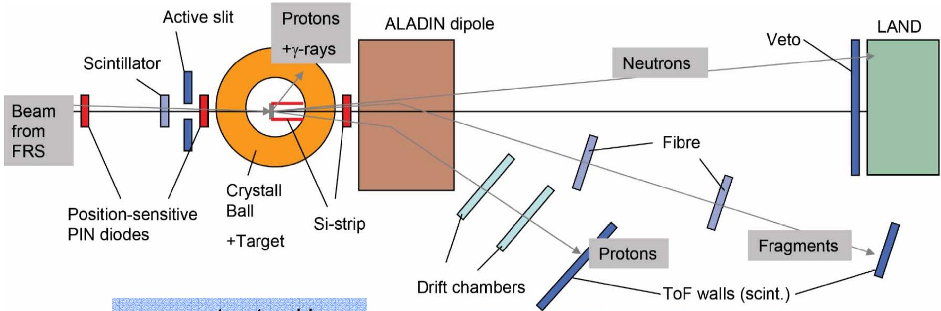
**new:** proton tracking around the target with Si-strip detectors
