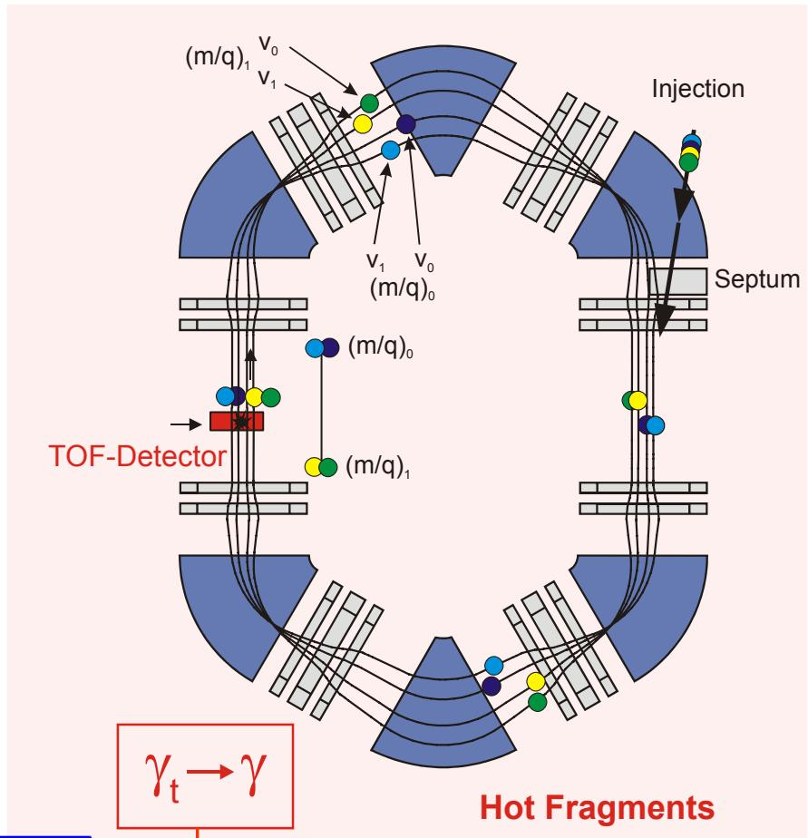
$$\frac{\Delta f}{f} = -\frac{1}{\gamma_t^2} \frac{\Delta(m/q)}{m/q} + \frac{\Delta v}{v} \left(1 - \frac{\gamma^2}{\gamma_t^2}\right)$$
