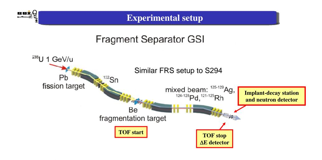
Assuming an incident intensity of  $2*10^9$  particles/spillTransmission to F2 ~ 8% $10^4$  ions/spill  $^{132}$ SnTransmission F2-F4 ~ 40%total implantation rate ~10 /s
