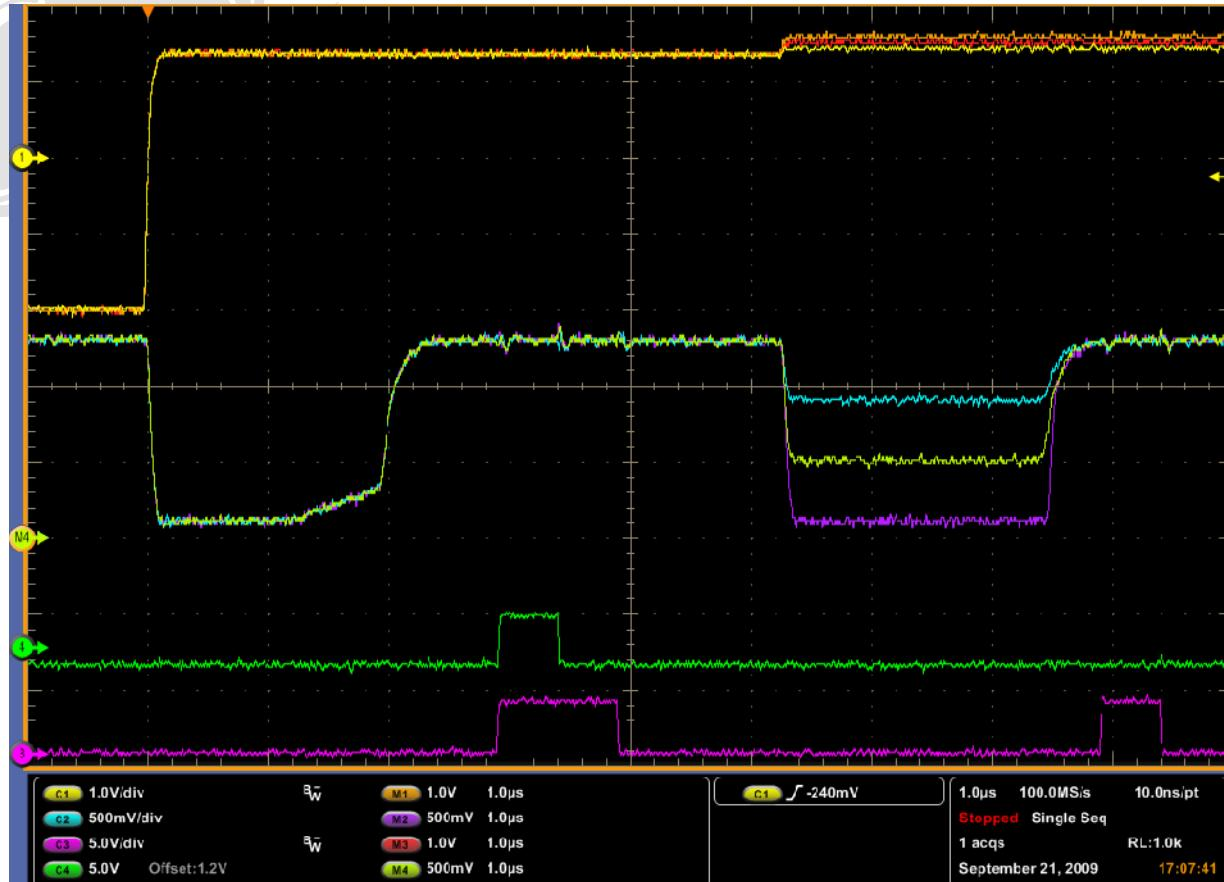
Fixed high-energy (HE) event (610pC) followed by three ME events (15pC, 30pC, 45pC): the ASIC recovers autonomously from the overload of the L-ME channel and the second event is read correctly.
