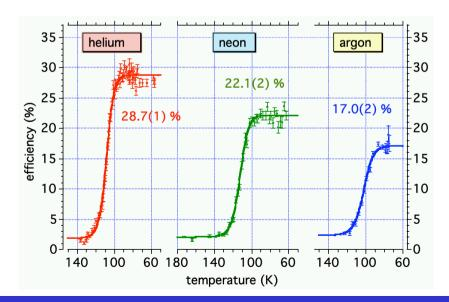
Transport efficiency of  $\alpha$ -decay recoil ions in a closed gas cell
