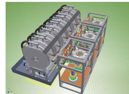
h=2 acceleration cavity for faster ramping
