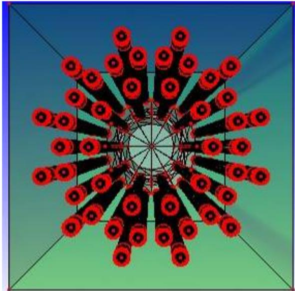
The detector has very high and flat efficiency (~60%) to minimise energy dependence
